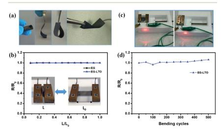
Fig. 2 Flexibility test of EG-LTO hybrids. (a) Flexibility of EG-LTO hybrid film. (b) Resistance variation of EG paper and EG-LTO hybrid under different bending states. (c) EG-LTO hybrid film connected a circuit at different bending states. (d) Resistance variation of EG-LTO hybrid after various bending cycles.
