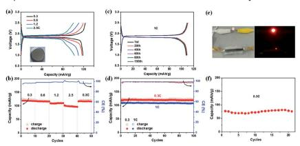
Fig. 4 Full-cell electrochemical performance of EG-LTO and EG-LFP. (a and b) Rate performance, (c and d) cycling stability and corresponding charge-discharge curves in coin cells. (e and f) An image of a pouch-type full cell with a transparent package and its battery performance at 0.3C
