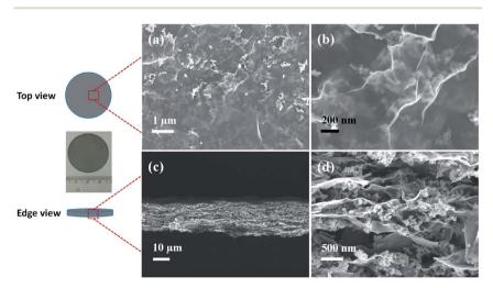
Fig. 1 SEM images of EG-LTO hybrid from top view (a and b) and edge view (c and d). Inset is an optical image of the EG-LTO hybrid film.
