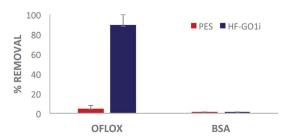
Fig. 10 Filtration of tap water spiked with 50 mg  $L^{-1}$  of ofloxacin and 10 g  $L^{-1}$  of BSA. Quantification by HPLC-UV analysis.
