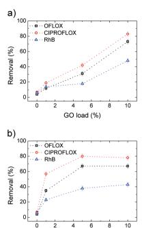
Fig. 8 Removal efficiency for OFLOX, Ciproflox and RhB vs. GO loading for (a) HF-GOe and (b) HF-GOi. The concentration (5 mg  $L^{-1}$ ), flow (15 mL min $^{-1}$ ) and fluxed volume (250 mL) of the contaminant solutions were the same for all tests. Filtration was performed by flowing water firstly passing through the GO layer, *i.e.* in–out for inner coated fibers and out–in for outer coated fibers.
