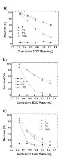
Fig. 9 Removal efficiency for Ciproflox (a), OFLOX (b) and RhB (c) for PES and increasing GO loading in HF-GOi. The cumulative initial mass is obtained with fixed concentration (5 mg L<sup>-1</sup>) and flow (15 mL min<sup>-1</sup>). Details are reported in Fig. S10. The curves for HF-GOe filters are shown in Fig. S11, ESI.†
