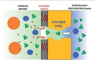
Fig. 12 Simplified working mechanism of HF-GO, allowing simultaneous filtration of BSA through PES and GO-promoted adsorption of OFLOX, Ciproflox and RhB. The GO layer does not cover all the pores, thus allowing EOC molecules to intercalate and nanoobjects to pass through the core—shell HF.
