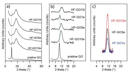
Fig. 5 (a) XRD patterns of HF-GO fibers and GO powder; (b and c) direct comparison of GO peaks. To allow a more direct comparison, in (b and c) the XRD signal due to background and polymer has been subtracted and in (c) a shift on the 2-theta scale was also applied.
