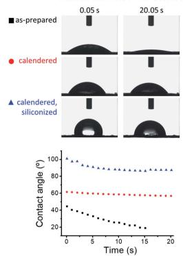
Fig. 6 Advancing contact angle measurements of 5 µL sessile water drops resting on samples of paper coated with ERG.
