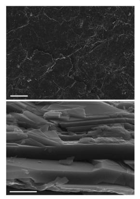
Fig. 2 Top: SEM micrograph of an ERG layer painted on paper. Bottom: View of a cut side surface. Scale bars: top, 100 μm; bottom, 2 μm.
