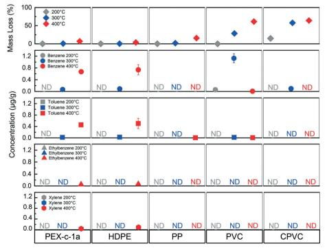
Fig. 3 Mean BTEX concentration after extracting each burned material at 200 °C, 300 °C, and 400 °C in water. The error bars reflect the standard deviation of the measurements (n = 3). If no error bars are visible, it indicates they were smaller than the symbol size. ND indicates the compound was not detected.
