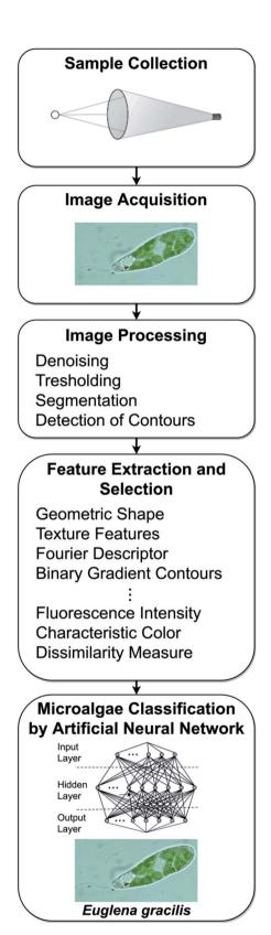
Fig. 1 The five steps of the automatic microalgae classification process by means of digital microscopy.
