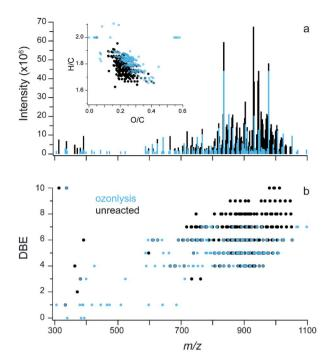
Fig. 4 Soft ionization mass spectra of unreacted (black) and ozonolysis (blue) samples. (a) ESI FT-ICR data with absolute intensity for CHO compounds in glass surface extracts, (b) DBE vs. m/z. The sample exposed to ozonolysis is shown as open circles in (b) to aid visualization
