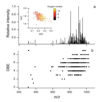
Fig. 2 Soft ionization mass spectra. (a) ESI FT-ICR data for CHO compounds in glass surface extracts, inset is the Van Krevelen plot with markers coloured by the number of oxygen atoms in the molecule; two molecules are off scale (see Fig. S3b†). (b) DBE vs. m/z for the
