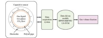
Fig. 12 Principle of CO<sub>2</sub> GVF measurement using capacitive sensors.<sup>27</sup>
