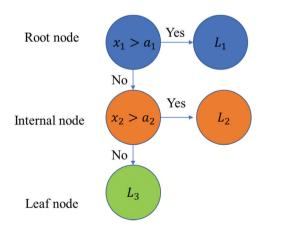
Fig. 13 Illustration of a CART. L denotes the leaf node (modified from Zhang et  $al.^{201}$ ).
