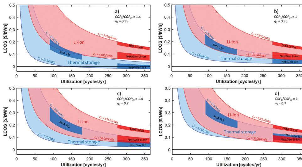
Fig. 4 LCOS comparison of TES + heat pump to EES + heat pump for four sets of TES baseline assumptions. (a) high  $COP_c/COP_{av}$ , high storage efficiency; (b) low  $COP_c/COP_{av}$ , high storage efficiency; (c) high  $COP_c/COP_{av}$ , low storage efficiency; (d) low  $COP_c/COP_{av}$ , low storage efficiency.
