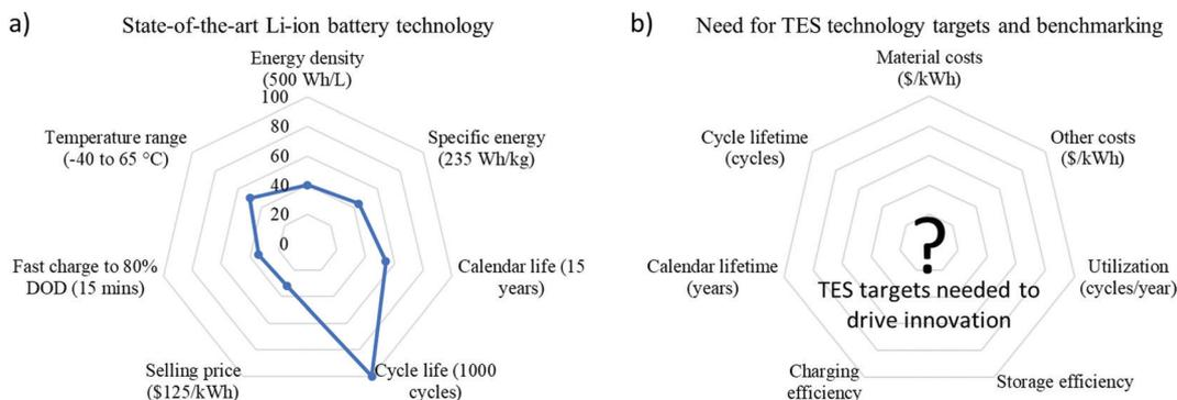
Fig. 6 (a) Comparison of state-of-the-art Li-ion technology with targets set by the USABC for all electric vehicles with a 200-mile range, adapted from Auston *et al.*<sup>62</sup> (b) There is a similar need for technology targets and benchmarking for TES applications in buildings.
