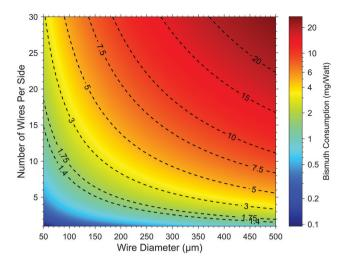
Fig. 13 Calculated bismuth consumption as a function of the number of wires per side and the wire diameter assuming a 3 µm coating of SnBi and cell efficiency of 25.11%
