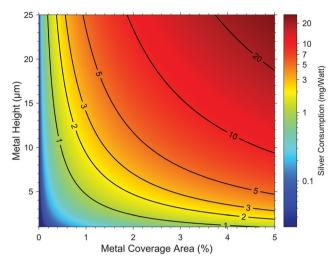
Fig. 5 Silver consumption as a function of printed metal coverage area and height in typical PERC solar cells. The assumed cell efficiency and the area are 23.83% and 210  $\times$  210 mm<sup>2</sup>. Contour lines represent different silver consumption levels.
