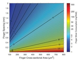
**Fig. 3** Finger silver consumption for 23.8% efficient PERC cells as a function of front finger spacing and finger cross-sectional area. The wafer area is assumed to be 210  $\times$  210 mm<sup>2</sup>. The hashed region has the finger silver consumption above the 2 mg W<sup>-1</sup> target. Contour lines represent different finger silver consumption levels.
