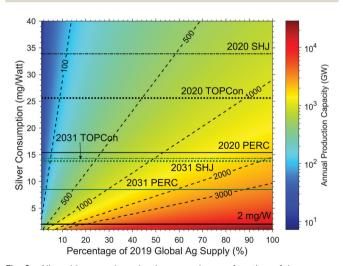
Fig. 2 Allowable annual production capacity as a function of the percentage of 2019 global silver supply that can be used in PV manufacturing and silver consumption in mg  $W^{-1}$ . Assumptions of efficiencies and silver consumption for PERC, TOPCon, and SHJ solar cells in 2020 and 2031 can be found in Table 2
