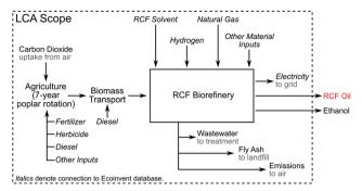
Fig. 9 LCA system boundary diagram, with connections to background LCI database indicated with italics
