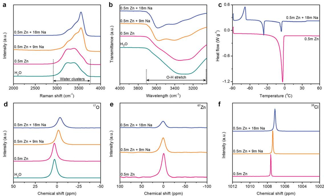
Fig. 2 Spectroscopic characterizations of the electrolytes. (a) Raman spectra, (b) FT-IR spectra, (c) DSC profiles, (d)  $^{17}\text{O}$  (water) NMR spectra, (e)  $^{67}\text{Zn}$  NMR spectra, and (f)  $^{35}\text{Cl}$  NMR spectra.
