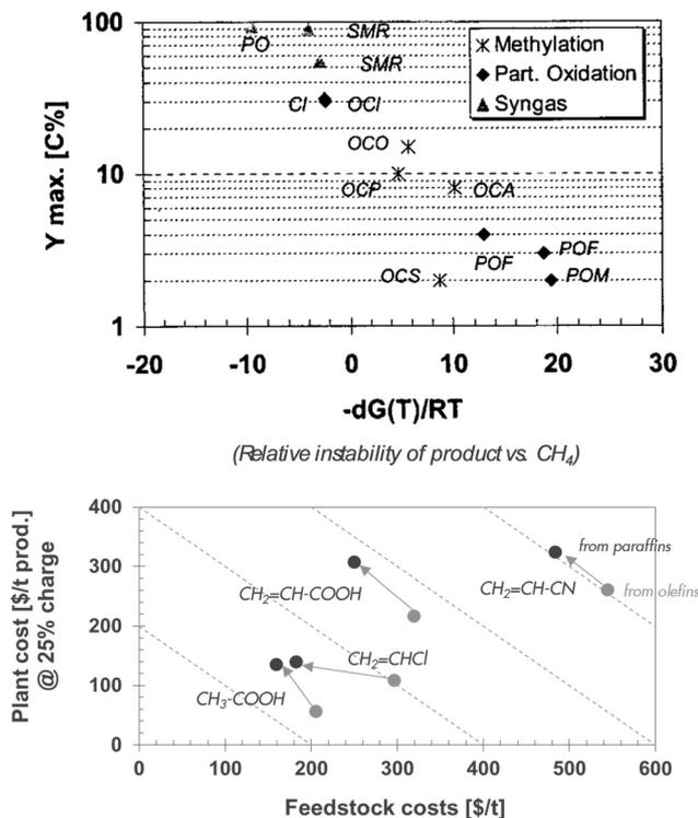
Fig. 3 Challenges in using natural gas. Top: thermodynamic limitation to yields in direct conversion of CH<sub>4</sub> (the acronyms are explained in the appendix).<sup>35</sup> Bottom: economic trade-off between feed and plant costs in direct oxidation of alkanes to chemical intermediates (black) vs. conventional olefin conversion (grey) (the diagonal dotted lines of the bottom figure represent the sum of feed cost and plant cost, the lion's share of the total manufacturing cost).<sup>36</sup>
