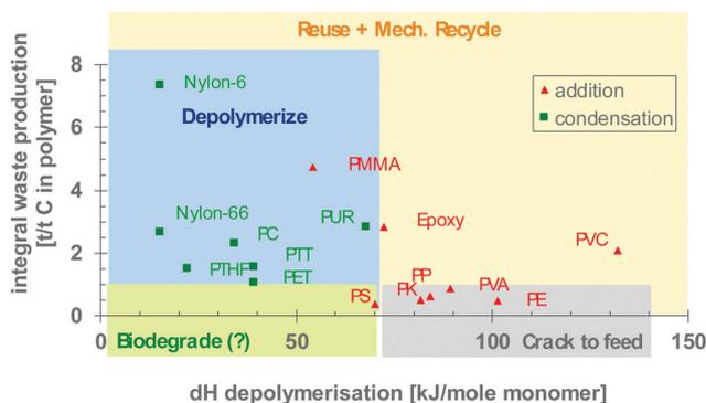
Fig. 9 Options for plastic recycling (adapted from Lange<sup>15</sup>).
