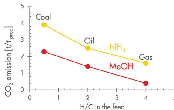
Fig. 6 Carbon intensity of fossil feedstocks for producing methanol and ammonia (adapted from Neelís<sup>68</sup>).
