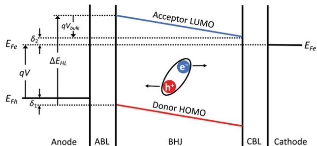
Fig. 1 Energy level diagram of an OPV under forward bias that is smaller than the open-circuit voltage. The hole quasi-Fermi energy,  $E_{\text{Fh}}$ , is pinned at  $\delta_1$  above the donor HOMO level on the anode side, while the electron quasi-Fermi energy,  $E_{\text{Fe}}$ , is at  $\delta_2$  below the acceptor LUMO level on the cathode side.
