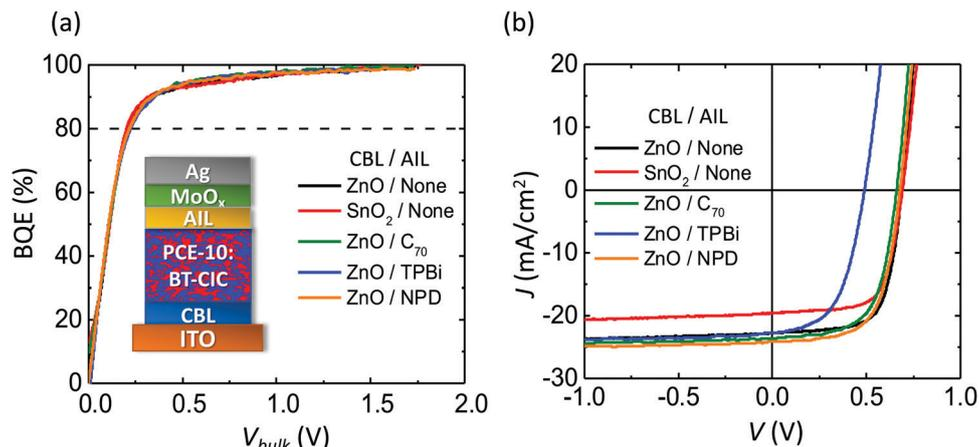
Fig. 6 (a) BQE– $V_{\text{bulk}}$  characteristics of OPVs with identical BHJs of PCE-10 as the donor and BT-C1C as the acceptor (1:1.5 by weight, 80 nm thick) and various cathode buffer layer (CBL)/AIL compositions. Inset: Device structure. (b)  $J$ – $V$  characteristics of devices in (a).
