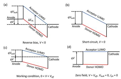
Fig. 2 (a) Energy level diagram of an OPV with ohmic contacts under reverse bias. (b) Energy level diagram of the OPV at short-circuit, (c) under solar cell working conditions, and (d) when there is no electric field across the BHJ.
