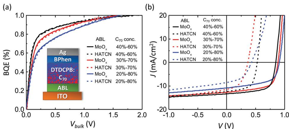
Fig. 5 (a) BQE– $V_{\text{bulk}}$  characteristics of DTDCPB: $C_{70}$  OPVs with gradient  $C_{70}$  concentrations from the anode to the cathode side (80 nm), and various anode buffer layers (ABLs). Inset: Device structure. (b) Current density–voltage ( $J$ – $V$ ) characteristics of devices in (a).
