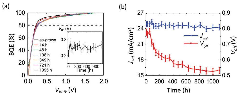
Fig. 10 (a) BQE- $V_{\text{bulk}}$  characteristics of a PCE-10:BT-CIC OPV with a self-assembled monolayer (C<sub>60</sub>-SAM) inserted between the BHJ and the ZnO layer under simulated AM 1.5G illumination. Inset:  $V_{80}$  vs. aging time. (b)  $V_{\text{off}}$  and  $J_{\text{sat}}$  vs. aging time.
