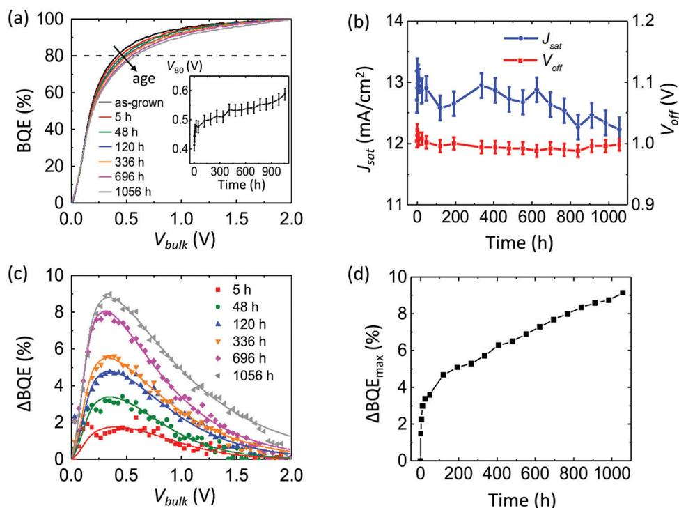
Fig. 7 (a) BQE– $V_{\text{bulk}}$  characteristics of a DBP:C<sub>70</sub> OPV aged under white light with an intensity equivalent to 27 suns. Inset:  $V_{80}$  vs. aging time. (b)  $V_{\text{off}}$  and  $J_{\text{sat}}$  vs. aging time. (c) Experimental (symbols) and fitted (lines) values of the decrease in BQE relative to the as-grown device ( $\Delta\text{BQE}$ ) vs.  $V_{\text{bulk}}$  at various aging times. (d) Maximum values of  $\Delta\text{BQE}$  vs. aging time.
