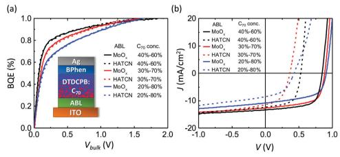
Fig. 5 (a) BQE- $V_{\text{bulk}}$  characteristics of DTDCPB:C<sub>70</sub> OPVs with gradient C<sub>70</sub> concentrations from the anode to the cathode side (80 nm), and various anode buffer layers (ABLs). Inset: Device structure. (b) Current density-voltage (J-V) characteristics of devices in (a).
