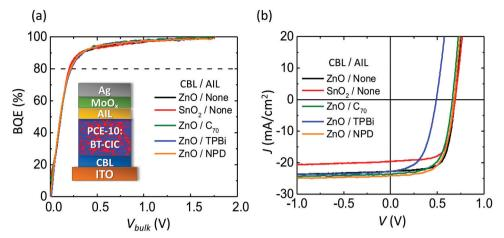
Fig. 6 (a) BQE-V<sub>bulk</sub> characteristics of OPVs with identical BHJs of PCE-10 as the donor and BT-CIC as the acceptor (1:1.5 by weight, 80 nm thick) and various cathode buffer layer (CBL)/AIL compositions. Inset: Device structure. (b) J-V characteristics of devices in (a).
