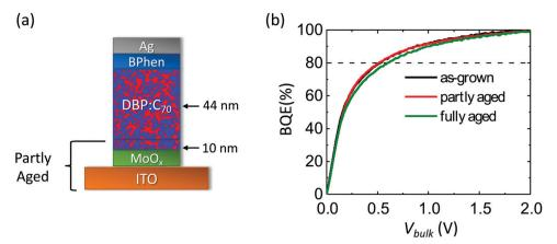
Fig. 8 (a) Structure of the partly aged and fully aged OPVs. The ITO layer,  $MOO_x$  layer and bottom 10 nm of the BHJ were aged under white light with an intensity equivalent to 27 suns for 17 days in the partly aged device. (b)  $BQE-V_{bulk}$  characteristics of the partly aged device, the as-grown device, and the fully aged device.
