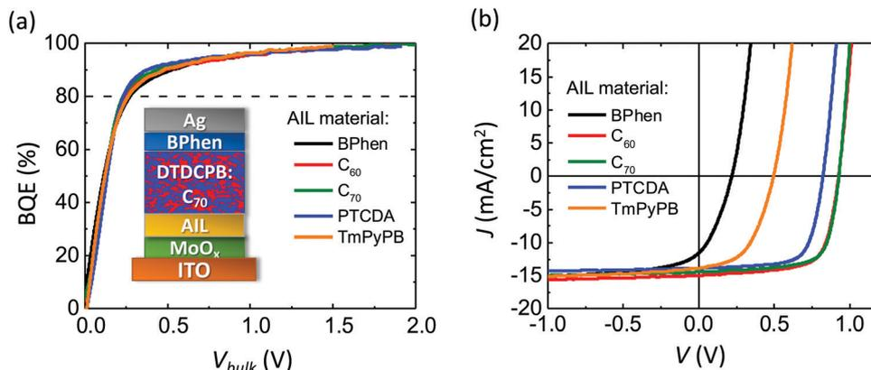
Fig. 4 (a) BQE– $V_{\text{bulk}}$  characteristics of OPVs with identical BHJs comprising DTDCPB as the donor and  $C_{70}$  as the acceptor (1 : 2 by volume, 80 nm thick) and various anode interface layers (AILs). Inset: Device structure. (b)  $J$ – $V$  characteristics of devices in (a).
