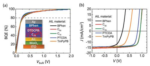
Fig. 4 (a) BQE $-V_{\text{bulk}}$  characteristics of OPVs with identical BHJs comprising DTDCPB as the donor and  $C_{70}$  as the acceptor (1:2 by volume, 80 nm thick) and various anode interface layers (AlLs). Inset: Device structure. (b) J-V characteristics of devices in (a).
