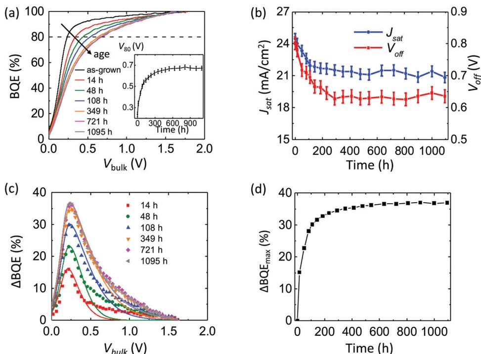
Fig. 9 (a) BQE– $V_{\text{bulk}}$  characteristics of an inverted OPV with a PCE-10:BT-CIC BHJ and a ZnO CBL aged under simulated AM 1.5G illumination. Inset:  $V_{80}$  vs. aging time. (b)  $V_{\text{off}}$  and  $J_{\text{sat}}$  vs. aging time. (c) Experimental (symbols) and fitted (lines) decrease in BQE ( $\Delta\text{BQE}$ ) vs.  $V_{\text{bulk}}$  vs. aging time. (d) The maximum values of  $\Delta\text{BQE}$  vs. aging time.
