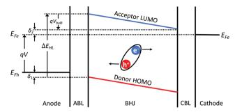
Fig. 1 Energy level diagram of an OPV under forward bias that is smaller than the open-circuit voltage. The hole quasi-Fermi energy,  $E_{\text{Fh}}$ , is pinned at  $\delta_1$  above the donor HOMO level on the anode side, while the electron quasi-Fermi energy,  $E_{\text{Fe}}$ , is at  $\delta_2$  below the acceptor LUMO level on the cathode side
