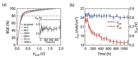
Fig. 10 (a) BQE- $V_{\text{bulk}}$  characteristics of a PCE-10:BT-CIC OPV with a self-assembled monolayer ( $C_{60}$ -SAM) inserted between the BHJ and the ZnO layer under simulated AM 1.5G illumination. Inset:  $V_{80}$  vs. aging time. (b)  $V_{off}$  and  $J_{sat}$  vs. aging time.
