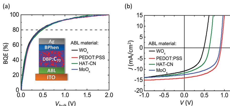
Fig. 3 (a) BQE- $V_{\text{bulk}}$  characteristics of OPVs with identical bulk heterojunction (BHJ) layers of DBP as the donor and C<sub>70</sub> as the acceptor (1:8 by volume, 54 nm thick), and various anode buffer layers (ABLs). Inset: Device structure. (b) Current density-voltage ( $J$ - $V$ ) characteristics of devices in (a).
