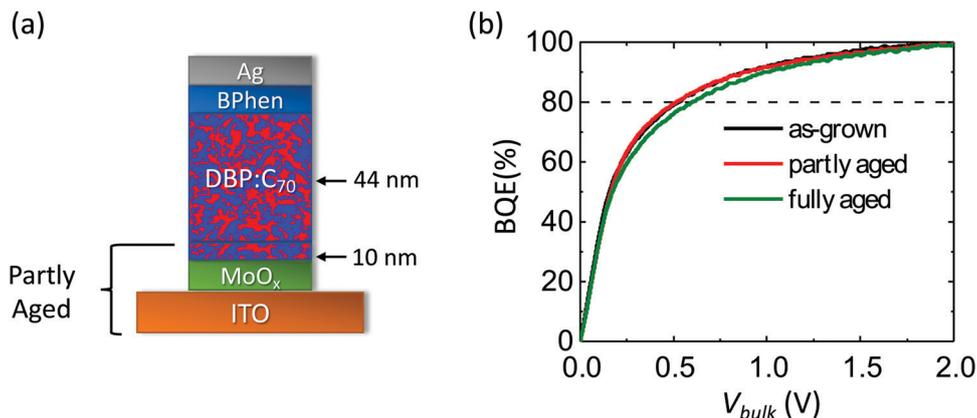
Fig. 8 (a) Structure of the partly aged and fully aged OPVs. The ITO layer, MoO<sub>x</sub> layer and bottom 10 nm of the BHJ were aged under white light with an intensity equivalent to 27 suns for 17 days in the partly aged device. (b) BQE– $V_{\text{bulk}}$  characteristics of the partly aged device, the as-grown device, and the fully aged device.
