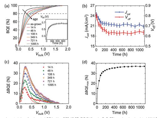
Fig. 9 (a) BQE-V<sub>bulk</sub> characteristics of an inverted OPV with a PCE-10:BT-CIC BHJ and a ZnO CBL aged under simulated AM 1.5G illumination. Inset:  $V_{80}$  vs. aging time. (b)  $V_{\text{off}}$  and  $J_{\text{sat}}$  vs. aging time. (c) Experimental (symbols) and fitted (lines) decrease in BQE ( $\Delta$ BQE) vs.  $V_{\text{bulk}}$  vs. aging time. (d) The maximum values of  $\Delta$ BQE vs. aging time.
