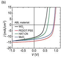
Fig. 3 (a) BQE-V<sub>bulk</sub> characteristics of OPVs with identical bulk heterojunction (BHJ) layers of DBP as the donor and C<sub>70</sub> as the acceptor (1:8 by volume, 54 nm thick), and various anode buffer layers (ABLs). Inset: Device structure. (b) Current density-voltage (J-V) characteristics of devices in (a).
