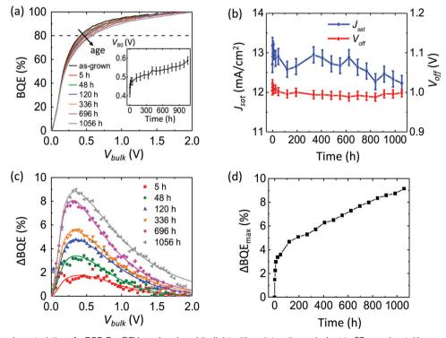
Fig. 7 (a) BQE- $V_{\text{bulk}}$  characteristics of a DBP: $C_{70}$  OPV aged under white light with an intensity equivalent to 27 suns. Inset:  $V_{80}$  vs. aging time. (b)  $V_{\text{off}}$  and  $J_{\text{sat}}$  vs. aging time. (c) Experimental (symbols) and fitted (lines) values of the decrease in BQE relative to the as-grown device ( $\Delta$ BQE) vs.  $V_{\text{bulk}}$  at various aging times. (d) Maximum values of  $\Delta$ BQE vs. aging time.
