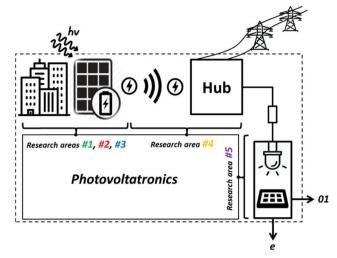
Fig. 6 A typical visual representation of photovoltatronics main energyinformation chain, including the five reported research areas. It graphically shows, how PV modules integrated into urban areas and equipped with integrated storage and electronics send energy wirelessly to an energy exchange hub, and how the energy flow continues to provide power for LEDs to send out information-based radiation modulated on visible light to be detected by a PV cell.
