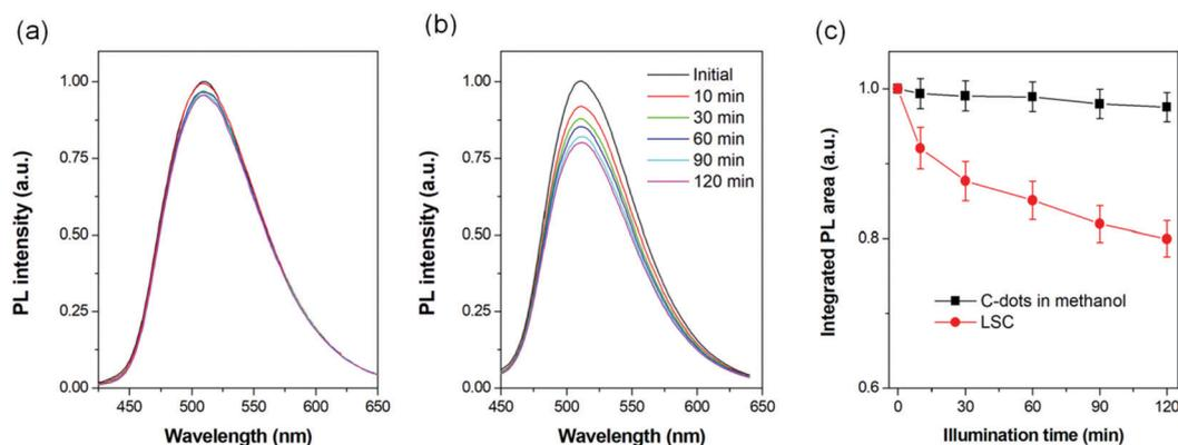
**Fig. 6** PL spectra of the C-dots dispersed in methanol (a) and in LSC (b) upon illumination. (c) The integrated PL area of the C-dots upon illumination. The  $400\text{-nm}$  illumination had an intensity of  $500 \text{ mW cm}^{-2}$ .
