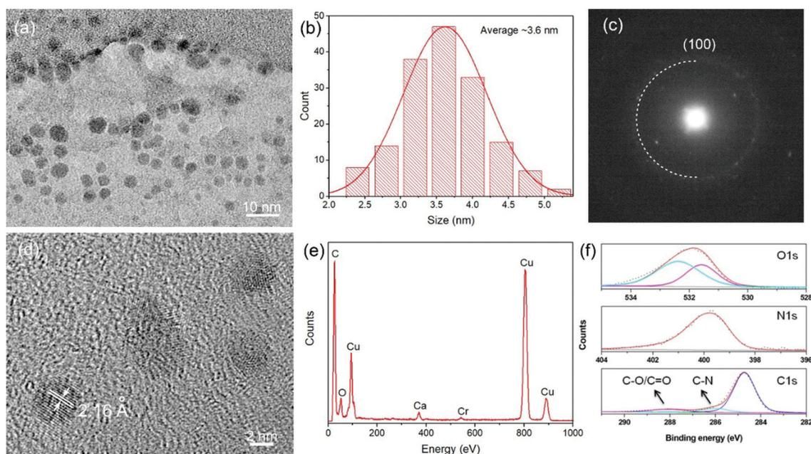
Fig. 1 Typical TEM image (a) and size distribution (b) of the C-dots synthesized *via* the vacuum heating approach. (c) SAED pattern and (d) HRTEM image of the C-dots. (e) EDS of the C-dots. (f) High-resolution XPS spectra of the C-dots.
