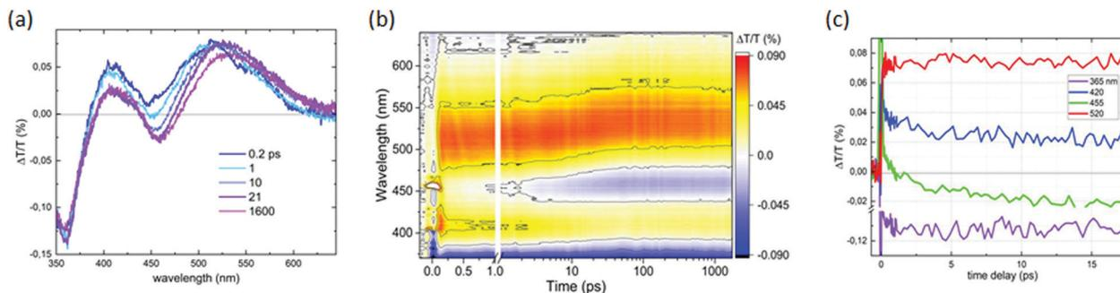
Fig. 3  $\Delta T/T$  spectra of C-dots produced by the space-confined vacuum-heating approach: (a) spectra for selected time delays, (b) map, (c) dynamics for selected wavelengths; pump@400 nm with fluence of  $6.5 \text{ mJ cm}^{-2}$ , pump and probe polarization are set at magic angle.
