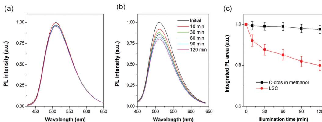
**Fig. 6** PL spectra of the C-dots dispersed in methanol (a) and in LSC (b) upon illumination. (c) The integrated PL area of the C-dots upon illumination. The 400-nm illumination had an intensity of 500 mW cm<sup>-2</sup>.
