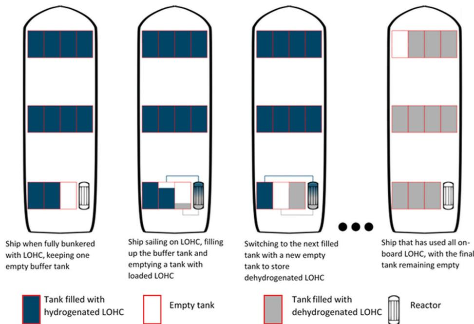
Fig. 5 Use of a buffer tank for LOHC fuel systems on board of a ship.
