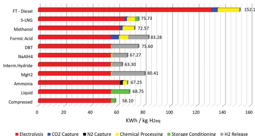
Fig. 3 Energy comparison for the storage requirements for the selected hydrogen storage carriers. The total sum of the values of these carriers is the total energy required (in kW h) to produce and store 1 kg of hydrogen (=33 kW h, LHV) with all the assumed product and energy losses.
