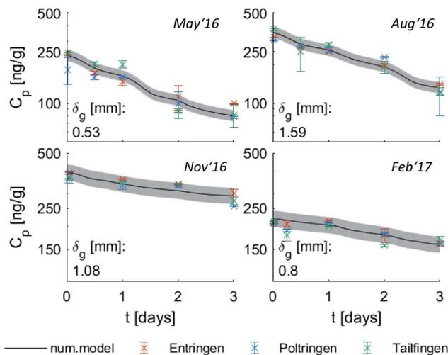
Fig. 1 Seasonal PRC-loss during the first year of monitoring, measured at each location and fitted (black solid line) based on measurements averaging over all locations. The air-side boundary layer thickness  $\delta_g$  was fitted for the average concentrations on PE. Error bars refer to triplicate samples at each location and the grey area indicates the standard deviation of the predicted concentration.
