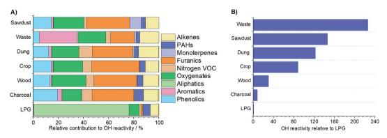
Fig. 6 OH reactivity of emissions from different fuel types with (A) relative contribution to OH reactivity and (B) total OH reactivity of fuel types at the top of flue relative to LPG, which is set to 1.
