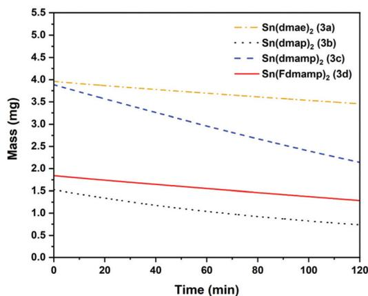
**Fig. 7** Isothermal plots at 70 °C of Sn(dmae)<sub>2</sub> (3a), Sn(dmap)<sub>2</sub> (3b), Sn(dmamp)<sub>2</sub> (3c) and Sn(Fdmamp)<sub>2</sub> (3d). Ar flow 20 mL min<sup>-1</sup>.
