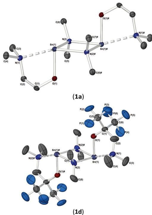
**Fig. 2** (a) The solid state molecular structures of [Sn{μ-NMe<sub>2</sub>}(dmae)<sub>2</sub>]<sub>2</sub> (**1a**), and (b) [Sn{μ-NMe<sub>2</sub>}(Fdmamp)<sub>2</sub>]<sub>2</sub> (**1d**). Thermal ellipsoids are shown at 50% probability. H-Atoms are omitted for clarity. The symmetry equivalent atoms are generated by the operator: # –X, 1 – Y, 1 – Z (**1a**) and #1 – X, 2 – Y, 1 – Z (**1d**).
