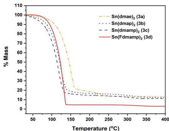
Fig. 6 Mass loss/temperature plots of  $[\text{Sn}\{\text{dmae}\}_2]$  (**3a**),  $[\text{Sn}\{\text{dmap}\}_2]$  (**3b**),  $[\text{Sn}\{\text{dmamp}\}_2]$  (**3c**) and  $[\text{Sn}\{\text{Fdmamp}\}_2]$  (**3d**). Ramp:  $5^\circ\text{C min}^{-1}$ , Ar flow  $20\text{ mL min}^{-1}$ .
