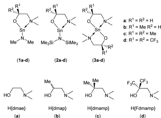
Fig. 1 The target hetero- (**1a–d** and **2a–d**) and homo-leptic Sn(II) systems (**3a–d**) derived from the aminoalcohol pro-ligands H{dmae} (**a**), H{dmamp} (**b**), H{dmamp} (**c**) and H{Fdmamp} (**d**) respectively.
