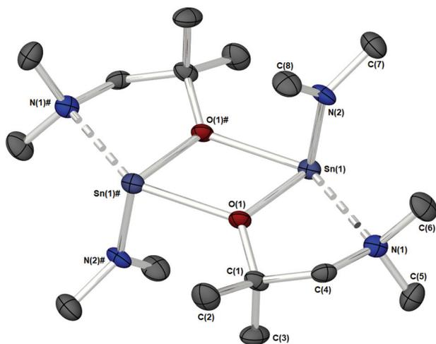
**Fig. 3** The solid state molecular structure of  $[\text{Sn}\{\mu\text{-dmamp}\}\{\text{NMe}_2\}_2]$  (**1c**). Thermal ellipsoids are shown at 50% probability. H-Atoms are omitted for clarity. The symmetry equivalent atoms are generated by the operator: #  $-X, 1 - Y, 1 - Z$ .
