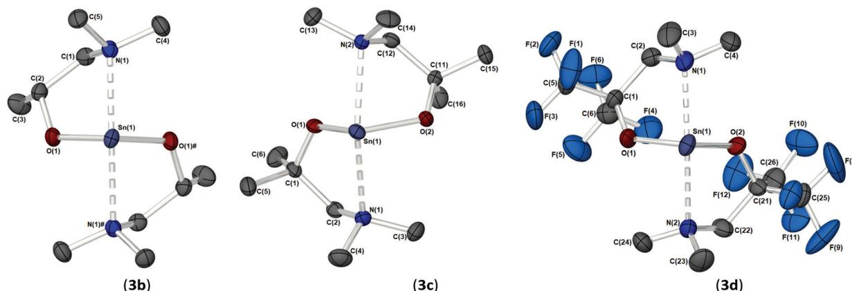
**Fig. 5** The solid-state molecular structures of (a) [Sn(dmap)<sub>2</sub>] (**3b**), (b) [Sn(dmamp)<sub>2</sub>] (**3c**) and (c) [Sn(Fdmamp)<sub>2</sub>] (**3d**). Thermal ellipsoids are shown at 50% probability and H-atoms are omitted for clarity. The symmetry equivalent atoms in **3b** are generated by the operator: # 1 – X, Y,  $\frac{1}{2}$  – Z.
