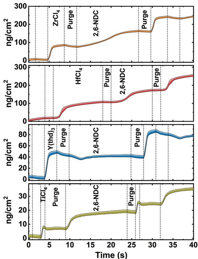
Fig. 3 Mass increase as a function of time measured *in situ* with QCM for Zr-NDC, Hf-NDC, Y-NDC and Ti-NDC. Inorganic precursor pulses and 2,6-NDC pulses are separated by inert gas (N<sub>2</sub>) purges. The shaded area represents the statistical variation during 16 cycles.
