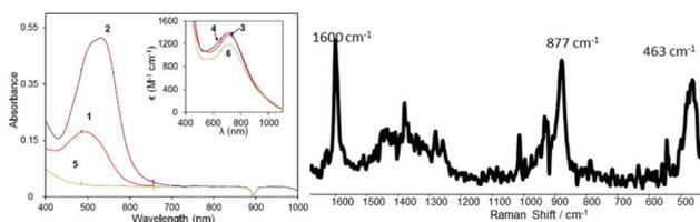
Fig. 2 (Left) UV-vis absorption spectra of  $\text{Fe}^{\text{II}}(\text{L}_{1,2,3})_3]^{2+}$  (**1**, **2**, **5**) in MeCN and their corresponding complexes  $[\text{Fe}_2^{\text{III}}(\mu\text{-O}_2)(\text{L}_{1,2,3})_2(\text{S})_2]^{4+}$  (**3**, **4** and **6**) generated by addition of 4 equiv.  $\text{H}_2\text{O}_2$  at 25 °C (inset). (Right) Raman spectrum of **6** at 785 nm generated from **5** (10 mM) by addition of 2 equiv.  $\text{H}_2\text{O}_2$ , with solvent signals subtracted.
