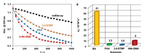
Fig. 5 Decay of absorbance of  $[\text{Fe}_2^{\text{III}}(\mu\text{-O}_2)(\text{L}_3)_2(\text{S})_2]$  (**6**) ( $\text{S}$  = solvent) at 705 nm in  $\text{CH}_3\text{CN}$  upon and in the presence of 4Me-DMA, 2,6-DTBP or PAA at 278 K with 2<sup>nd</sup> order rate constants for comparison.
