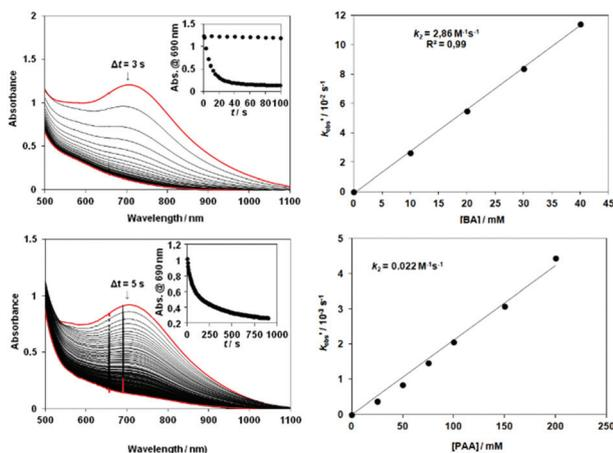
Fig. 3 Reaction of  $[\text{Fe}_2^{\text{III}}(\mu\text{-O}_2)(\text{L}_3)_2(\text{S})_2]$  (**6**) ( $\text{S}$  = solvent) with benzaldehyde. UV-vis absorption spectrum over time (inset absorbance at 705 nm over time) following addition of (Upper) benzaldehyde and (Lower) phenylacetaldehyde to *in situ* generated **6** and corresponding plots of  $k'_{\text{obs}} (= k_{\text{obs}} - k_{\text{selfdecay}})$  versus [aldehyde] at 278 K.
