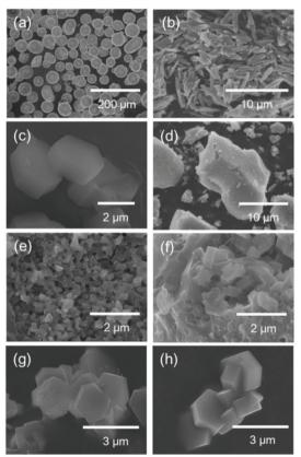
Fig. 5 PXRD patterns and SEM images of experiments using ball milling for the treatment of reagents and zeolite seed crystals prior to steam treatment. SEM images show the precursors silica powder (a), sodium aluminate (b) and ZSM-5 seed crystals (c), as well as materials obtained after milling (d) and final products after 6 h (e), 12 h (f), and 18 h (g) of steam treatment. Reproduced from ref. 83 with permission from Wiley-VCH, copyright 2017.
