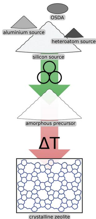
**Fig. 2** Schematic illustration of mechanochemical pre-treatment of reagents prior to crystallisation.
