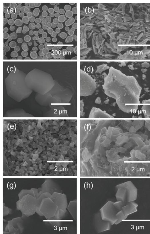
**Fig. 5** PXRD patterns and SEM images of experiments using ball milling for the treatment of reagents and zeolite seed crystals prior to steam treatment. SEM images show the precursors silica powder (a), sodium aluminate (b) and ZSM-5 seed crystals (c), as well as materials obtained after milling (d) and final products after 6 h (e), 12 h (f), and 18 h (g) of steam treatment. Reproduced from ref. 83 with permission from Wiley-VCH, copyright 2017.
