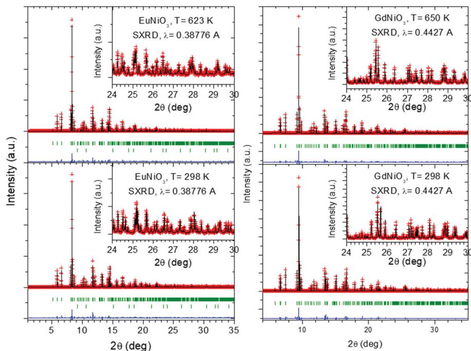
Fig. 2 Rietveld plots from the SXRDX data of  $\text{EuNiO}_3$  (left column) at RT and 623 K and  $\text{GdNiO}_3$  (right column, at RT and 650 K), corresponding to the structural refinements in the orthorhombic  $Pbnm$  space group in all cases. The insets show a close up of the high-angle region, highlighting the quality of the fit. The second series of Bragg reflections for  $\text{EuNiO}_3$  correspond to a minor impurity of NiO.
