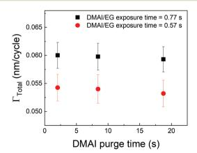
**Fig. 9**  $\Gamma_{\text{Total}}$  as a function of DMAI purge time. Unlike the observed decrease in  $\Gamma_{\text{Total}}$  with respect to TMA purge time, the DMAI purge time seems to have a negligible effect on  $\Gamma_{\text{Total}}$ .
