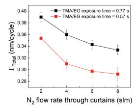
**Fig. 8**  $\Gamma_{Total}$  as a function of N<sub>2</sub> flow through the gas curtains. In these experiments, the partial pressures and exposure times of both TMA and EG were kept constant while only the N<sub>2</sub> flow through the four curtains was varied from 2 to 8 slm (0.5 to 4 slm per curtain).
