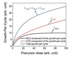
Fig. 3 A schematic showing different contributions in the total growth-per-cycle. The total GPC ( $\Gamma_{\text{Total}}$ ) could be seen as a result of contributions from the surface MLD reactions ( $\Gamma_{\text{CVD}}$ ).
