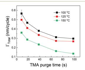
Fig. 6 Effect of deposition temperature on the decrease of  $\Gamma_{\mathrm{Total}}$  with TMA purge time.
