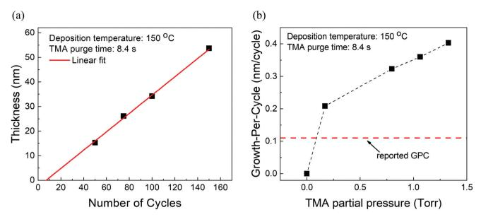
Fig. 2 (a) Measured film thickness vs. the number of cycles. The GPC is  $\sim$ 0.36 nm per cycle with an x-intercept of 8 cycles. (b) Growth-per-cycle vs. the partial pressure of TMA. In these experiments, the partial pressure of EG was kept constant at 0.5 Torr and a timing sequence of (0.77, 8.4, 0.77, 2) was used. The GPC shows no signs of saturation and even at the lowest TMA partial pressure of 0.17 Torr, it is already higher than previously reported GPC.<sup>15</sup>
