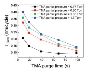
Fig. 4  $\Gamma_{Total}$  as a function of TMA purge time. In these experiments conducted at 150 °C, the EG dose, its purge time and TMA exposure time were kept constant while the TMA purge time was varied. For each TMA partial pressure,  $\Gamma_{\mathrm{Total}}$  decreases with increasing TMA purge time and upon a long enough purge stabilizes at a steady-state value equal to  $\Gamma_{\rm MLD}$ .
