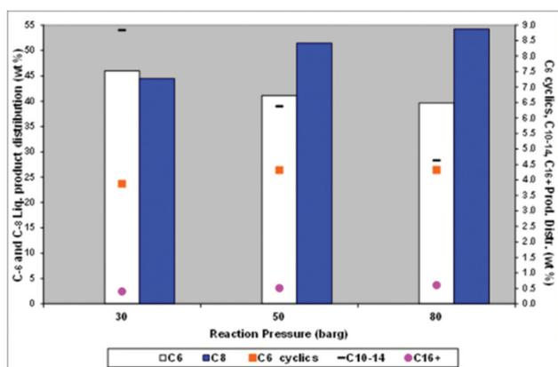
**Fig. 3** Effect of reaction pressure on product selectivity.
