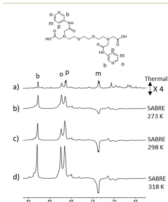
**Fig. 3** Partial single scan  $^1\text{H}$  NMR spectra of the aromatic region of a sample containing (a) thermally polarised  $[\text{IrCl}(\text{COD})(\text{IMes})]$  (2.5 mM) and  $S_{2m}$  (4 equiv.) in 0.6 mL of methanol- $d_4$  (b)–(d) the same sample after shaking with 3 bar  $\text{pH}_2$  at 65 G for 10 seconds after being left in a thermostatically controlled water bath at (b) 273 K (c) 298 K and (d) 318 K for 60 seconds prior to  $\text{pH}_2$  shaking.
