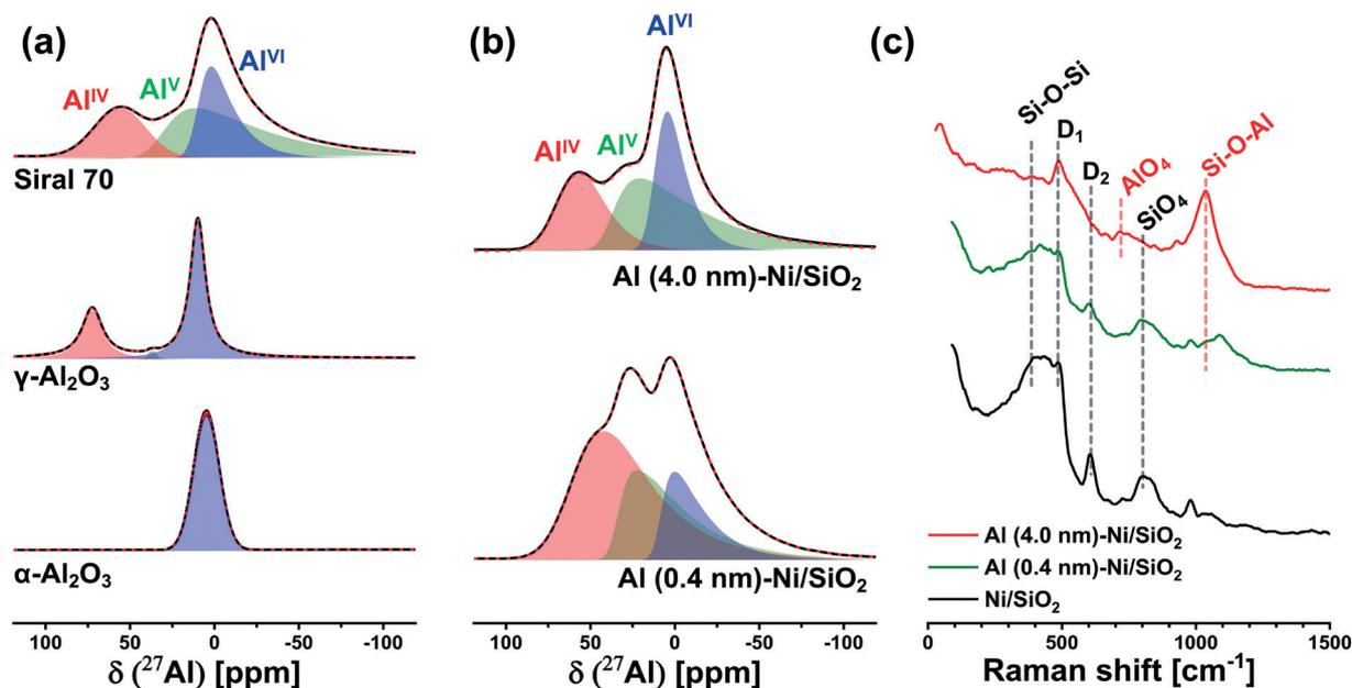
Fig. 3 Characterization of the interaction between silica and alumina: solid-state <sup>27</sup>Al-NMR of (a)  $\alpha$ -Al<sub>2</sub>O<sub>3</sub>,  $\gamma$ -Al<sub>2</sub>O<sub>3</sub>, and aluminosilicate Siral 70 references; and (b) calcined Al (0.4 nm)-Ni/SiO<sub>2</sub> and Al (4.0 nm)-Ni/SiO<sub>2</sub>. (c) Raman spectra of calcined Ni/SiO<sub>2</sub>, Al (0.4 nm)-Ni/SiO<sub>2</sub>, and Al (4.0 nm)-Ni/SiO<sub>2</sub>.
