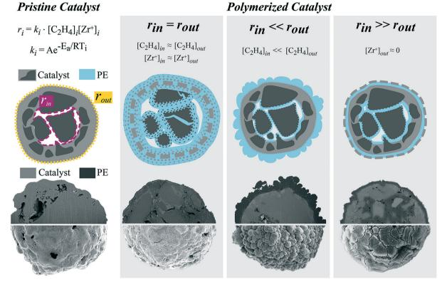
Fig. 8 Schematic of fragmentation modes experimentally observed for a metallocene-based ethylene polymerization catalyst supported on a silica support. Every experimentally observed catalyst particle fragmentation pattern can be described by the ratio between the rate of ethylene polymerization at the sites in the macropore walls in the core of the catalyst particle  $(r_{in})$  and the rate at the sites on the outer surface of the catalyst particle  $(r_{out})$ .
