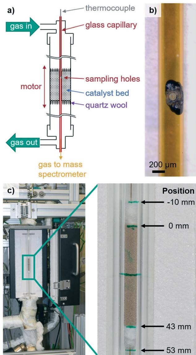
**Fig. 1** Scheme of the setup for simultaneous acquisition of gas phase concentration and temperature profiles along fixed catalyst beds (a), light microscope image of the glass capillary used for local sampling showing the laser drilled sampling holes ( $\varnothing = 50 \mu\text{m}$ ) with black marking for alignment during mounting (b), and photo of the setup with zoom in onto the catalyst bed with inserted sampling capillary and selected position indications (c).
