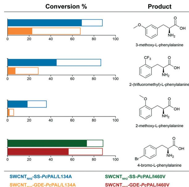
Fig. 8 Ammonia addition reactions of cinnamic acid derivatives catalyzed by site-specifically and non-specifically immobilized engineered *PcPAL* variants L134A and I460V. The color filled and empty bars represent the conversion values after 4 h and 20 h reaction times, respectively.
