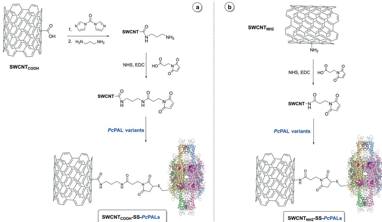
**Fig. 3** Site-controlled covalent immobilization of *PcPAL* on the a) SWCNT<sub>COOH</sub> and b) SWCNT<sub>NH<sub>2</sub></sub> supports.
