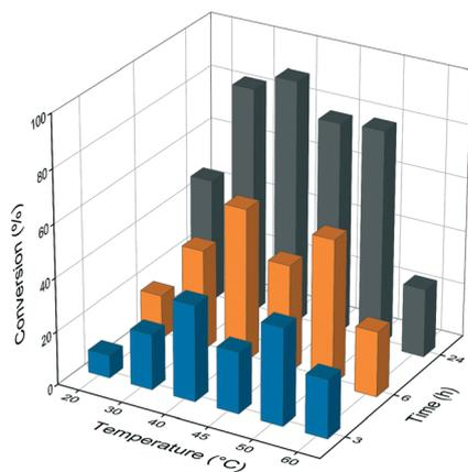
Fig. 7 Effect of temperature on the conversion values of the ammonia addition reaction of *trans*-cinnamic acid, using the optimal reaction medium (3 M  $\text{NH}_2\text{CO}_2\text{NH}_4$ ) and biocatalyst load (0.12 mg enzyme per mg support). Samples were taken at different reaction times (3, 6 and 24 hours respectively).
