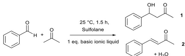
Fig. 9 The aldol reaction catalysed by binary alkoxide ionic liquids.<sup>69</sup>
