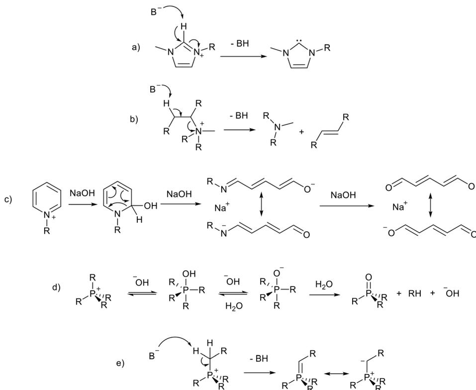
Fig. 2 Base catalysed decomposition of an imidazolium cation,  $B^-$  represents an external base or a basic anion (a),<sup>20</sup> Hofmann elimination of an acyclic ammonium cation (b),<sup>22</sup> ring opening decomposition of a pyridinium cation (c),<sup>23,24</sup> and formation of a phosphine oxide (d)<sup>25,26</sup> and phosphorus ylide (e)<sup>27</sup> from a phosphonium ionic liquid. Kekulé structures are drawn for clarity.
