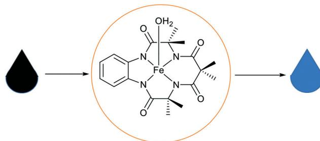
Fig. 26 A representation of water purification using Fe-TAML entrapped in basic ionic liquid silica materials.<sup>115</sup>
