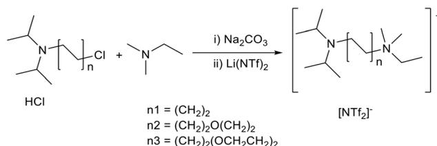
Fig. 5 The synthesis of Hunig's base containing ionic liquids.<sup>37</sup>
