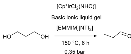
Fig. 25 The hydrogen transfer initiated dehydration of 1,3-propanediol promoted by a basic ionic liquid gel. 111
