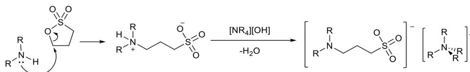
Fig. 10 An example of the synthesis of ionic liquids containing neutral amine anions.<sup>75</sup>
