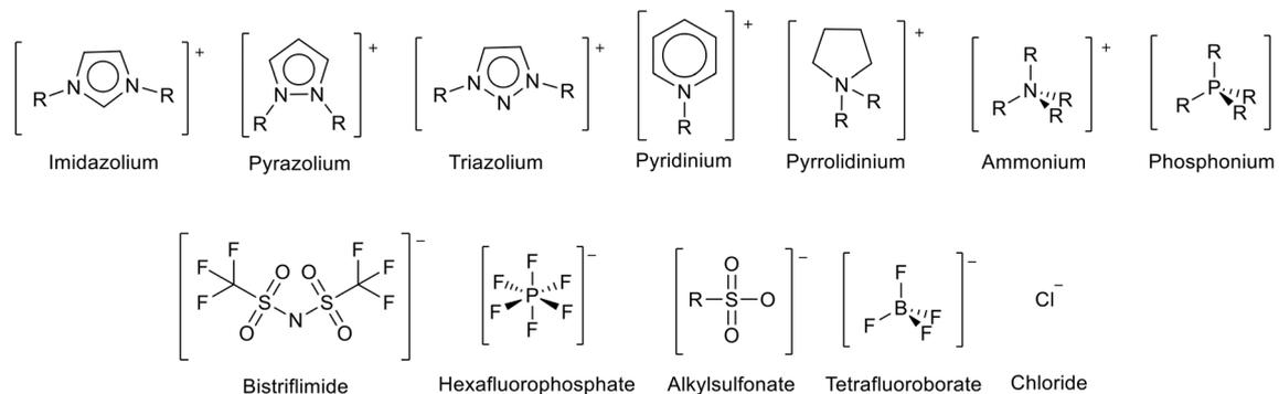
**Fig. 1** Some common cations and anions used to prepare ionic liquids.  $\text{PF}_6^-$  and  $\text{BF}_4^-$  have fallen out of general use due to concerns over their relative instability through hydrolysis to produce  $\text{HF}$ .<sup>5-7</sup>
