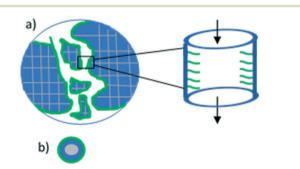
Fig. 24 a) A representation of ionic liquid tethered to mesoporous silica, and the diffusion of the substrate through the SILP pores. b) A representation of ionic liquid coated on a magnetic silica nanoparticle. Blue is silica, grey is  $CoFe_2O_4$  and green is ionic liquid. 106
