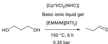
Fig. 25 The hydrogen transfer initiated dehydration of 1,3-propanediol promoted by a basic ionic liquid gel.<sup>111</sup>
