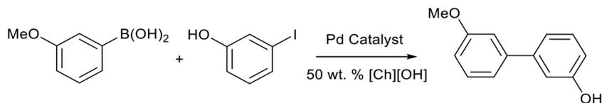
Fig. 16 The palladium catalysed Suzuki cross-coupling reaction between 3-methoxyphenylboronic acid and 3-iodophenol promoted by choline hydroxide.<sup>84</sup>
