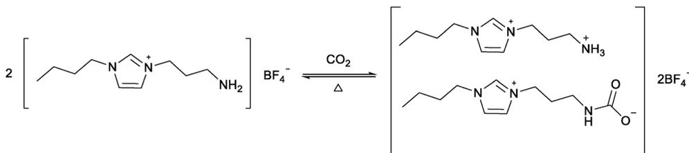
Fig. 17 The reaction between CO<sub>2</sub> and an amine functionalised ionic liquid proposed by Davis and co-workers.<sup>14</sup>
