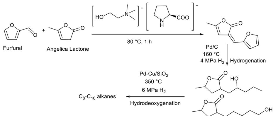
Fig. 12 Generation of fuel alkanes by the [Ch][Pro] catalysed aldol condensation between furfural and angelica lactone followed by hydrogenation and hydrodeoxygenation.<sup>78</sup>
