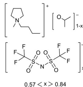
Fig. 8 The structure of binary alkoxide ionic liquids ( $[Pyrr_{1,4}][NTf_2]_x[O^iPr]_{1-x}$ ).<sup>69</sup>
