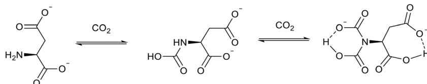
Fig. 18 CO<sub>2</sub> capture by the [Asp]<sup>-</sup> anion of [P<sub>6,6,6,14</sub>]<sub>2</sub>[Asp].<sup>91</sup>
