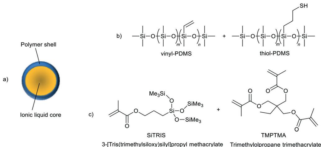
Fig. 27 A representation of an ionic liquid microcapsule as prepared by Stolaroff *et al.* (a), and the components of the different polymer shell materials (b and c).<sup>118</sup>
