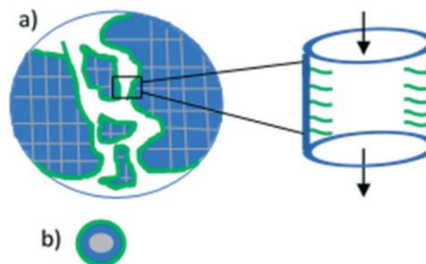
Fig. 24 a) A representation of ionic liquid tethered to mesoporous silica, and the diffusion of the substrate through the SILP pores. b) A representation of ionic liquid coated on a magnetic silica nanoparticle. Blue is silica, grey is  $CoFe_2O_4$  and green is ionic liquid.<sup>106</sup>
