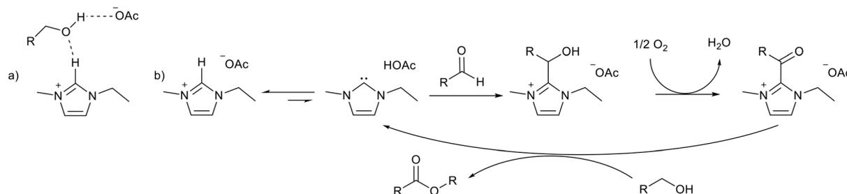
Fig. 14 a) Hydrogen bonding between [EMIM][OAc] and an alcohol substrate. b) Activation of an aldehyde by an NHC formed from [EMIM][OAc] leading to esterification.<sup>82</sup>
