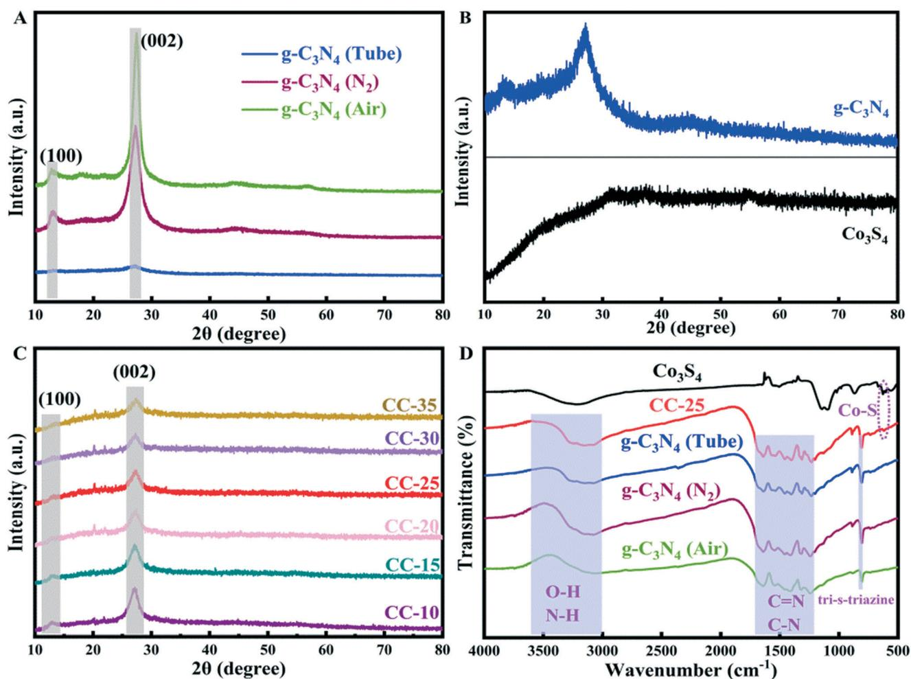
Fig. 1 XRD patterns of (A)  $g\text{-C}_3\text{N}_4$  (prepared using different methods), (B)  $\text{Co}_3\text{S}_4$  and  $g\text{-C}_3\text{N}_4$  tube, (C) CC- $x$  ( $x = 10, 15, 20, 25, 30, 35$ ), and (D) FT-IR spectra of  $g\text{-C}_3\text{N}_4$  (prepared using different methods),  $\text{Co}_3\text{S}_4$ , and CC-25.
