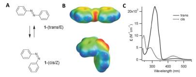
Fig. 13 (A) *E* (*trans*) and *Z* (*cis*) structural configurations of the azobenzene molecules. (B) Corresponding electrostatic potentials. Red indicates negative potential and blue indicates a positive potential. (C) Electronic absorption spectra for the *trans* (solid line) and *cis* (dotted line) configurations. Adapted from Beharry *et al.*, *Chem. Soc. Rev.*, 2011, **40**, 4422–4437, with permission from The Royal Society of Chemistry.<sup>137</sup>
