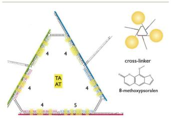
Fig. 12 Triangular assembly of gold nanoparticles, obtained by intercalation of 8-methoxypsoralen. The DNA template was designed to have twenty-five 5'-TA-3' sites as suitable positions for intercalation and subsequent crosslinking, resulting in stable formation of triangular assemblies. Reprinted from Ohshiro et al., Chem. Commun., 2010, 46, 6132-6134 with permission from The Royal Society of Chemistry. 131
