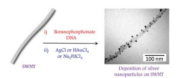
Fig. 34 Schematic illustration of single-walled carbon nanotube and TEM image of silver nanoparticles assembly on BP-DNA functionalised singlewalled carbon nanotubes. Reprinted from Chem. Mater. 2017, 29(5), 2239–2245, Copyright © 2017 American Chemical Society. 239
