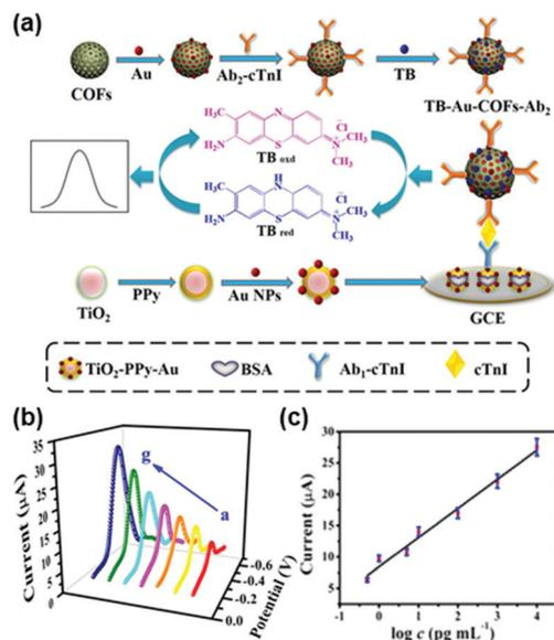
Fig. 25 (a) Schematic illustration of the sandwich-type electrochemical immunosensor. (b) SWV current responses with increasing cTnI concentrations from  $0.5 \text{ pg mL}^{-1}$  to  $10.0 \text{ ng mL}^{-1}$ . (c) Calibration curve of the immunosensor for the detection of different concentrations of cTnI.<sup>277</sup> Adapted with permission from ref. 277. Copyright 2018, Elsevier.
