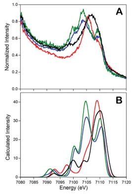
Fig. 4 Experimental (A) and calculated (B) valence-to-core XES spectra of compounds **6** (-), **9** (-), [L'FeCl]<sub>2</sub> (-), and [(L)Fe(N<sub>2</sub>)Fe(L)] (-). The feature at  $\sim$ 7100 eV is a key feature to determine the degree of dinitrogen activation. Reprinted with permission from ref. 69. Copyright (2013) American Chemical Society.
