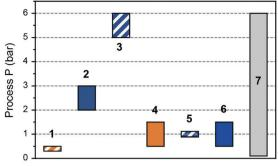
Fig. 6 Overview of PDH processes conditions. Ranges of temperature (left) and pressure (right) used in the CATOFIN (1), Oleflex (2), Uhde STAR (3), FBD Yarsintez-Snamprogetti (4), Linde-BASF PDH (5), FLOTU/Tsinghua (6), and SABIC (7). Stripes fill: cyclic operation; solid fill: continuous operation; orange: Cr-based catalyst; blue: Pt-based catalyst; grey: Pt or Cr-based catalysts.
