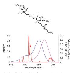
Fig. 3 Cyanine dye absorbance (blue), overlapping the Eu spectral output, and dye emission (purple), minimising overlap with [EuL<sup>9</sup>] emission (red), (MeOH, 295 K).
