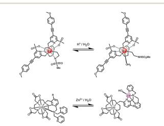
Scheme 6 The speciation at Eu in each complex changes reversibly following addition of acid (upper) or metal ion (lower), with dissociation of a nitrogen donor(s) and replacement by water. 116-119
