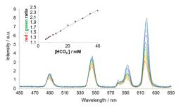
**Fig. 8** Time-gated spectral data showing the variation of emission for  $[EuL^{22}]^{3+}/[TbL^{22}]^{3+}$  following addition of bicarbonate ( $\lambda_{\rm exc}$  365 nm, 10 μs time gate, pH 7.4, 295 K, 0.1 M NaCl, 0.4 mm human serum albumin, 2.3 mM lactate, 0.13 mM citrate, 1 mM HPO<sub>4</sub><sup>2-</sup>, 1 mM ATP). The inset shows the red/green ratio change with increasing bicarbonate concentration. Adapted with permission from ref. 122. Copyright (2012) Wiley-VCH. <sup>122</sup>
