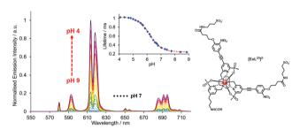
Fig. 12 pH Variation of europium emission of  $[EuL^{23}]^{2-}$  ( $\lambda_{exc}$  332 nm, 295 K, 0.1 M NaCl); showing the variations of the europium emission intensity and lifetime ( $\lambda_{exc}$  332 nm,  $\lambda_{em}$  613 nm) with a p $K_a$  value of 6.18(03). Reproduced with permission from the Royal Society of Chemistry. 125
