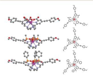
Fig. 5 Increased steric shielding of the Ln centre from vibrational quenching as the ligand carboxylate is replaced by P-Me and P-Ph phosphinate groups, increases the europium emission lifetime; (upper to lower:  $\tau^{Eu}$  (MeOH) = 0.99, 1.18 and 1.30 ms). Adapted with permission from ref. 23. Copyright (2014) Wiley-VCH.<sup>23</sup>
