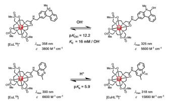
Scheme 4 (upper) Reversible attack by hydroxide modifies the sensitiser constitution, switching off Eu emission; (lower) N-protonation reduces  $k_{\rm eT}$ with a three-fold Eu intensity enhancement associated with suppression of photoinduced electron transfer. 14
