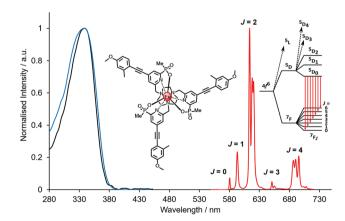
Fig. 2 Absorption (blue), excitation and emission spectra of [EuL<sup>9</sup>], showing the five major transitions in the visible region from the <sup>5</sup>D<sub>0</sub> Eu excited state (295 K, 0.1 M NaCl). Adapted with permission from the Royal Society of Chemistry.<sup>24</sup>
