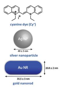
**Fig. 12** Molecular structure of an excitonic system based on a widely used cyanine dye, namely, 1,1'-diethyl-2,2'-cyanine iodide and plasmonic systems based on Ag NPs and Au NRs.<sup>15</sup> Dimensions of Au NP and Au NR used in Table 1 are indicated in this figure.
