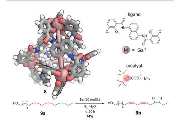
Fig. 7 Raymond and co-workers' regioselective hydrogenation catalysed by a non-covalently bound rhodium-phosphine complex. Colours: C grey, H white, Ga dark salmon (shown as spheres), N blue, O red.
