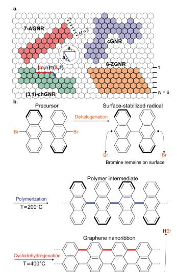
Fig. 1 (a) Various GNR types and their classification. (b) Schematic overview of on-surface GNR fabrication for the case of a 7-AGNR.
