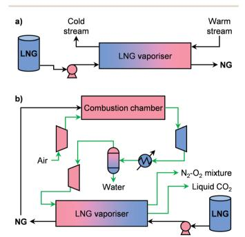
Fig. 10 (a) Scheme of a cold utilization plant that utilizes the heat of vaporisation of LNG to cool down a desired stream. (b) Flowsheet of a small-scale process for the generation of electricity and for cryogenic CO2 capture that uses LNG as fuel and cold source.
