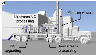
Fig. 16 Schematic representation of (a) a plant-on-wheels installed at the NG extraction site and of (b) its interior for decentralised NG upgrading
