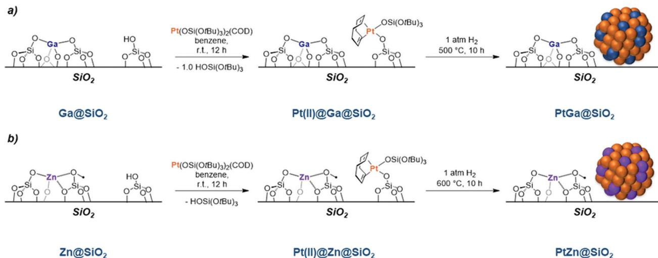
**Scheme 9** (a) Depiction of synthetic procedure employed for the generation of PtGa alloyed nanoparticles supported on Ga-doped silica using an SOMC/TMP approach; and (b) depiction of synthetic procedure employed for the generation of sub-nanometric PtZn alloyed nanoparticles on zinc-doped silica using an SOMC/TMP approach.
