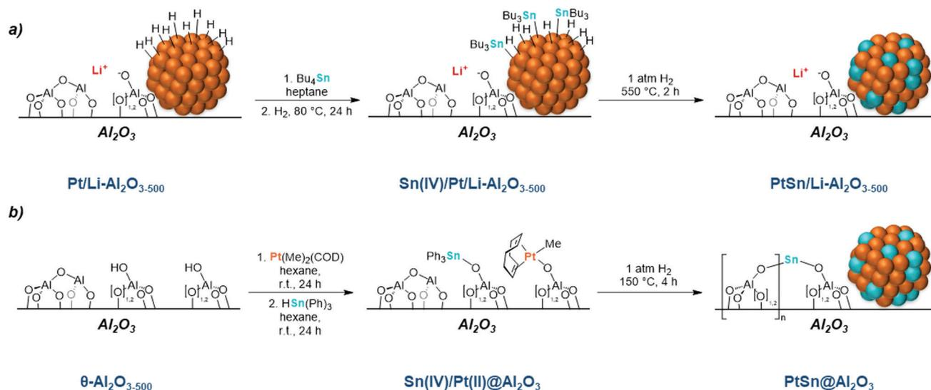
**Scheme 8** (a) Depiction of synthetic procedure employed for the generation of PtSn alloyed nanoparticles supported on Li-doped alumina using an SOMC metal functionalisation approach; and (b) depiction of synthetic procedure employed for the generation of PtSn alloyed nanoparticles on tin-doped  $\theta$ -alumina using an SOMC/TMP approach ( $n = 1, 3$ ).
