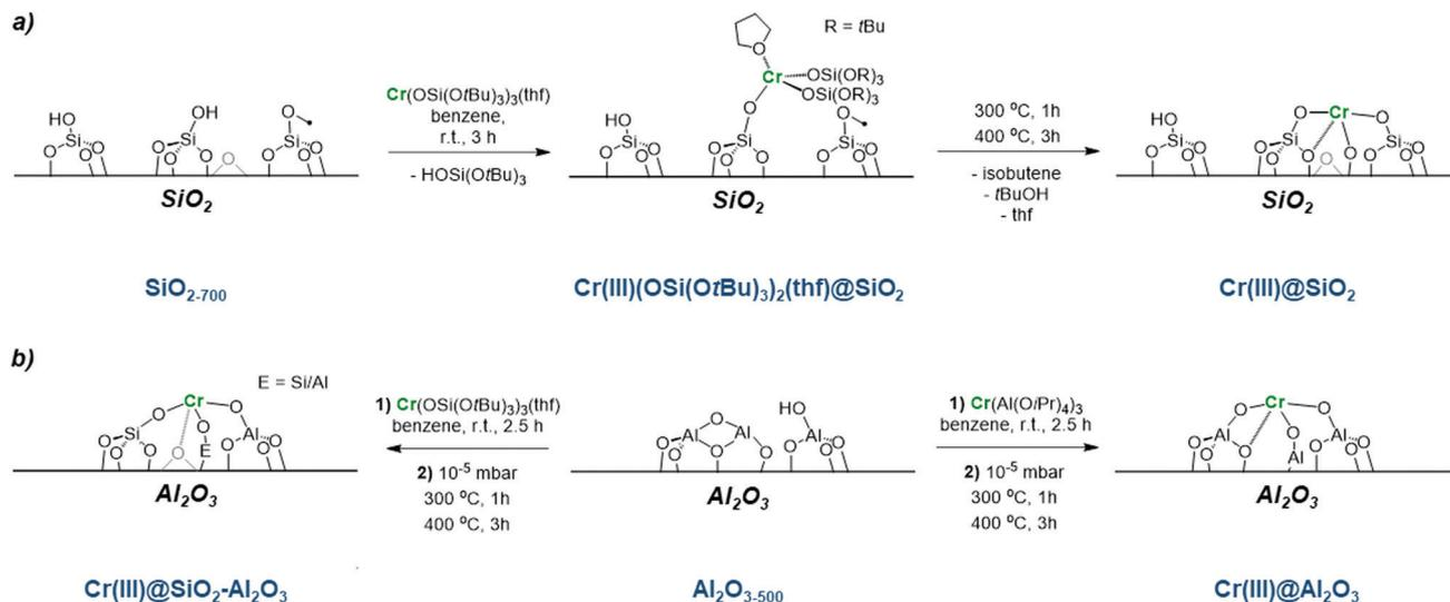
**Scheme 3** Isolated Cr<sup>III</sup> sites prepared using an SOMC/TMP approach (a) synthesis of Cr<sup>III</sup> single sites on SiO<sub>2</sub> partially dehydroxylated at 700 °C; and (b) SiO<sub>2</sub>-Al<sub>2</sub>O<sub>3</sub> and Al<sub>2</sub>O<sub>3</sub>.
