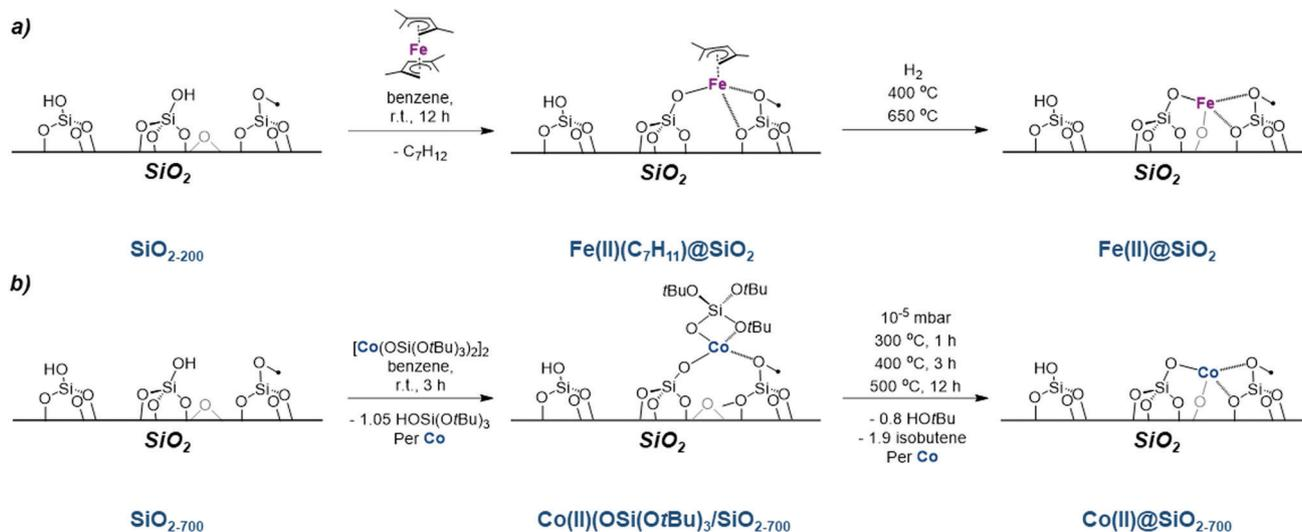
**Scheme 7** Preparation of silica supported  $\text{Fe}^{\text{II}}$  and  $\text{Co}^{\text{II}}$  isolated sites for PDH, (a) SOMC approach for the preparation of supported  $\text{Fe}^{\text{II}}$  single sites using bis-2,4-dimethylpentadienide iron(II) as molecular precursor; and (b) preparation of  $\text{Co}^{\text{II}}$  single sites for propane dehydrogenation prepared using a combined SOMC/TMP approach.
