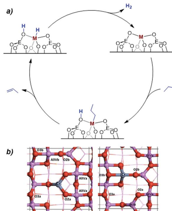
**Scheme 4** (a) Proposed non-redox mechanism for the dehydrogenation of light alkanes over M<sup>III</sup> isolated sites (M = Cr & E = Si or Al; or M = Ga & E = Si); and (b) structure of model tri- and tetra-coordinated Cr<sup>III</sup> sites on Al<sub>2</sub>O<sub>3</sub>. Reproduced from ref. 43 with permission from American Chemical Society, copyright 2016.
