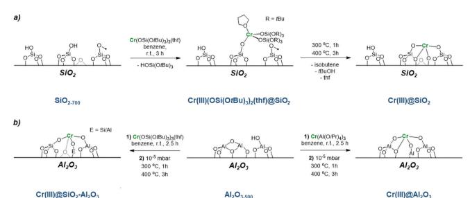
Scheme 3 Isolated  $Cr^{|||}$  sites prepared using an SOMC/TMP approach (a) synthesis of  $Cr^{|||}$  single sites on  $SiO_2$  partially dehydroxylated at 700 °C; and (b)  $SiO_2 - Al_2O_3$  and  $Al_2O_3$ .
