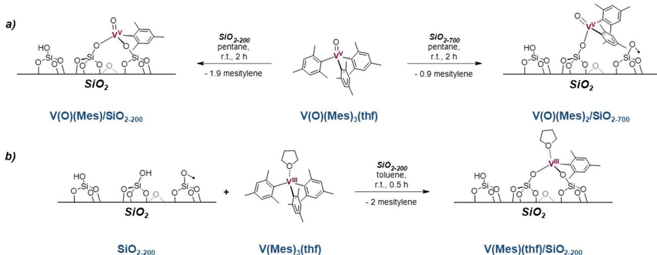
**Scheme 6** Preparation of silica supported  $\text{V}^{\text{III}}$  and  $\text{V}^{\text{V}}$  aryl complexes for PDH, (a) SOMC approach for the preparation of monopodal and bipodal supported  $\text{V}^{\text{V}}$  single sites employed in vanadium catalysed propane dehydrogenation; and (b) preparation of  $\text{V}^{\text{III}}$  single sites for propane dehydrogenation prepared using an SOMC approach.
