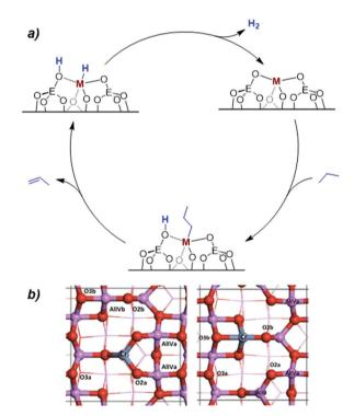
**Scheme 4** (a) Proposed non-redox mechanism for the dehydrogenation of light alkanes over  $M^{III}$  isolated sites (M = Cr & E = Si or Al; or M = Ga & E = Si); and (b) structure of model tri- and tetra-coordinated  $Cr^{III}$  sites on  $Al_2O_3$ . Reproduced from ref. 43 with permission from American Chemical Society, copyright 2016.
