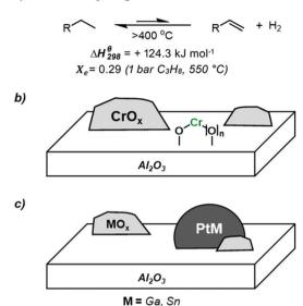
Scheme 1 (a) Dehydrogenation of light alkanes (thermodynamic constraints, equilibrium conversion of propane at 1 bar and 550 °C; (b) general structure of CATOFIN®-type catalysts (CrO<sub>x</sub>/Al<sub>2</sub>O<sub>3</sub>), and (c) general structure of platinumbased catalysts for the dehydrogenation of light alkanes (PtM/MO<sub>x</sub>/Al<sub>2</sub>O<sub>3</sub>).
