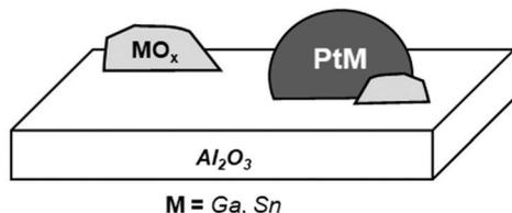
**Scheme 1** (a) Dehydrogenation of light alkanes (thermodynamic constraints, equilibrium conversion of propane at 1 bar and 550 °C); (b) general structure of CATOFIN<sup>®</sup>-type catalysts (CrO<sub>x</sub>/Al<sub>2</sub>O<sub>3</sub>), and (c) general structure of platinum-based catalysts for the dehydrogenation of light alkanes (PtM/MO<sub>x</sub>/Al<sub>2</sub>O<sub>3</sub>).
