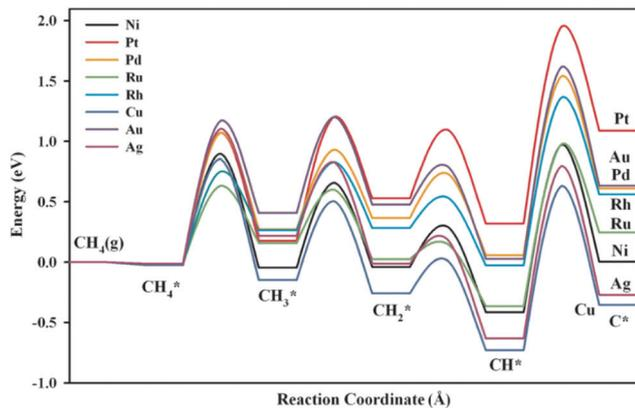
Fig. 12 Potential energy diagrams for methane dissociation on Ni-based bimetallic surfaces. The chemisorbed H atoms required to balance adsorption states have been omitted to simplify the notation.<sup>167</sup> Reproduced from ref. 167 with permission from AIP Publishing, copyright 2012.
