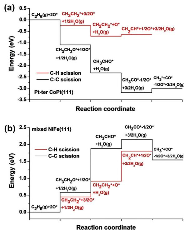
Fig. 25 DFT calculated energy profiles of reforming and ODH of ethane on (a) Pt-terminated CoPt(111) and (b) mixed FeNi(111).<sup>323</sup> Reproduced from ref. 323 with permission from Elsevier, copyright 2016.
