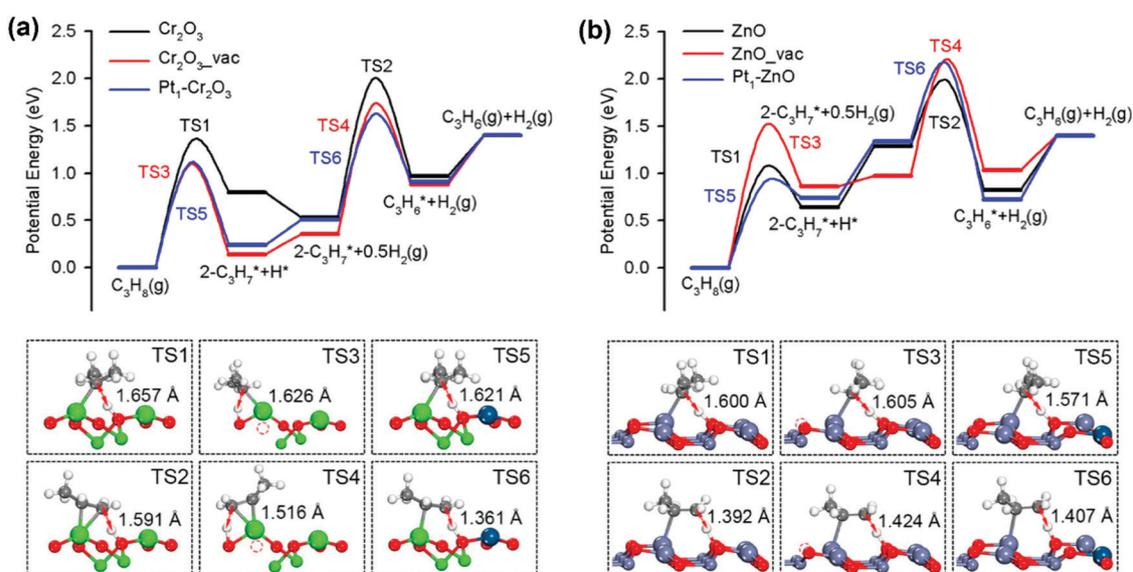
Fig. 38 Energy profiles for PDH on pristine, oxygen-deficient, and Pt-doped (a) Cr<sub>2</sub>O<sub>3</sub> and (b) ZnO surfaces. All the potential energies are referenced to gas-phase propane.<sup>405</sup> Reproduced from ref. 405 with permission from the American Chemical Society, copyright 2019.
