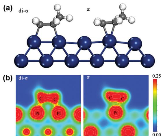
Fig. 27 (a) Adsorption modes of propylene on Pt surfaces.<sup>357</sup> Reproduced from ref. 357 with permission from Elsevier, copyright 2014. (b) The valence charge densities calculated for different propylene adsorption modes.<sup>349</sup> Reproduced from ref. 349 with permission from Elsevier, copyright 2010.
