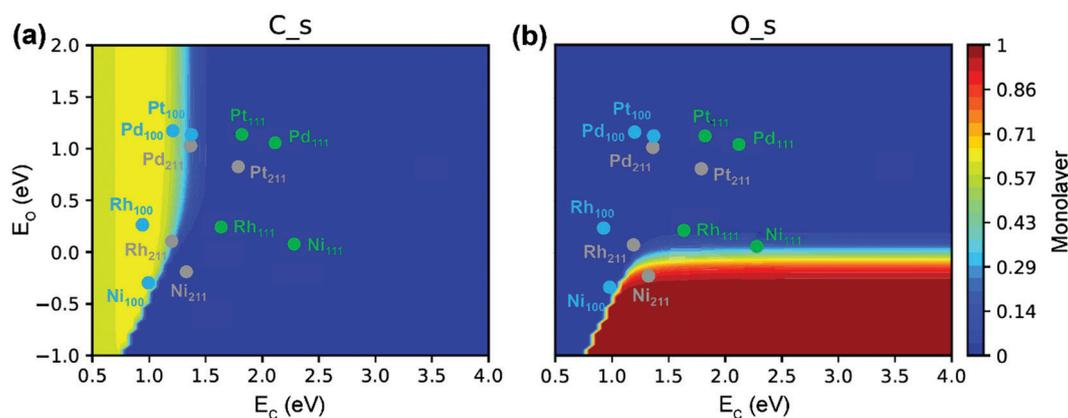
**Fig. 11** (a)  $\text{O}^*$  and (b)  $\text{C}^*$  site coverages as functions of C- and O-metal formation energies in SRM. Reaction conditions: 773 K, 1 bar, 18.2%  $\text{CH}_4$ , 63.6%  $\text{H}_2\text{O}$ , 18.2%  $\text{H}_2$ .<sup>89</sup> Adapted from ref. 89 with permission from the American Chemical Society, copyright 2020.
