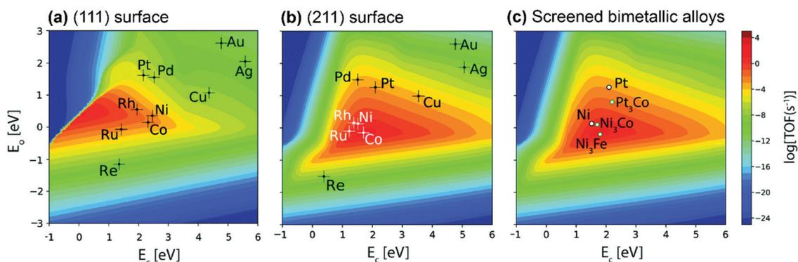
Fig. 26 Elementary reaction rate for oxygen assisted ethane dehydrogenation (C<sub>2</sub>H<sub>6</sub> + O → C<sub>2</sub>H<sub>5</sub> + OH) over the (a) (111) surface and (b) (211) surface of transition metal catalysts; and (c) screened alloy candidates.<sup>328</sup> Reproduced from ref. 328 with permission from the Royal Society of Chemistry, copyright 2020.
