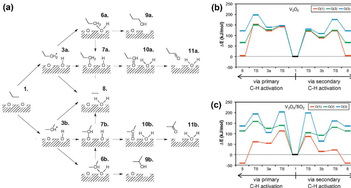
Fig. 35 (a) Investigated pathways for propane oxidation over the vanadia surface; the corresponding energy diagrams for propane oxidation to propylene on (b)  $V_2O_5$  and (c)  $V_2O_5/TiO_2$ .<sup>403</sup> Reproduced from ref. 403 with permission from Elsevier, copyright 2012.
