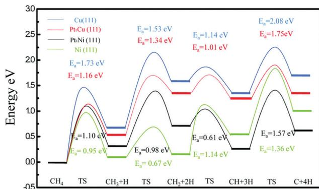
Fig. 17 Comparison of methane dissociation reaction pathways on Pt<sub>1</sub>Cu(111) and Pt<sub>1</sub>Ni(111) surfaces.<sup>231</sup> Reproduced from ref. 231 with permission from the Centre National de la Recherche Scientifique (CNRS) and the Royal Society of Chemistry, copyright 2020.
