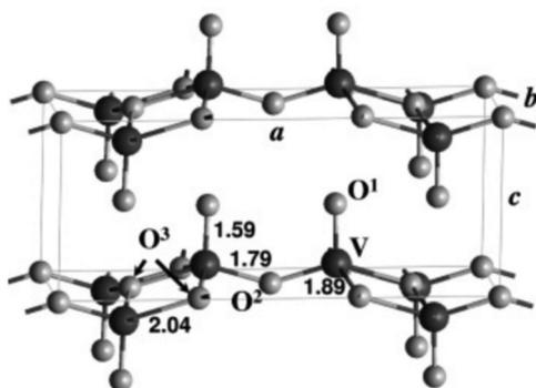
Fig. 33  $V_2O_5$  bulk surface.<sup>408</sup> *a*, *b*, and *c* of the orthorhombic unit cells are parallel to the (100), (010), and (001) directions, respectively. V atoms are depicted as the white circles and O atoms as the smaller gray circles.  $O_1$ ,  $O_2$ , and  $O_3$  denote the single, 2-fold, and 3-fold coordinated oxygen atoms, respectively. Bond lengths in Å. Reproduced from ref. 408 with permission from the American Chemical Society, copyright 2005.
