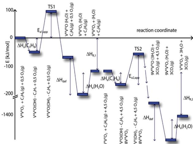
Fig. 37 Energy profile for propane ODH (left) and rate determining step of propane combustion over  $\text{VO}_x/\text{Al}_2\text{O}_3$  catalysts.<sup>15</sup> Reproduced from ref. 15 with permission from the American Chemical Society, copyright 2014.
