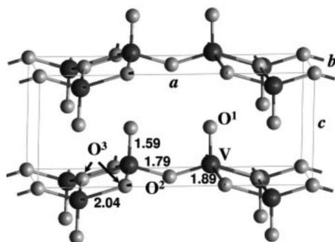
Fig. 33  $V_2O_5$  bulk surface.<sup>408</sup> *a*, *b*, and *c* of the orthorhombic unit cells are parallel to the (100), (010), and (001) directions, respectively. V atoms are depicted as the white circles and O atoms as the smaller gray circles.  $O_1$ ,  $O_2$ , and  $O_3$  denote the single, 2-fold, and 3-fold coordinated oxygen atoms, respectively. Bond lengths in Å. Reproduced from ref. 408 with permission from the American Chemical Society, copyright 2005.
