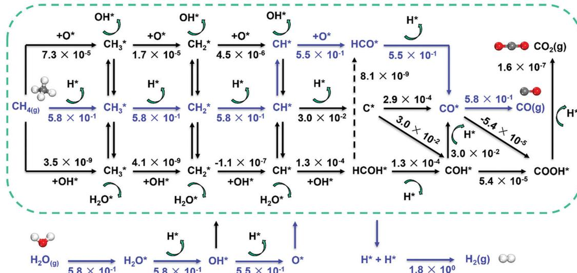
Fig. 7 Reaction network for SRM over Ni catalyst and estimated net turnover frequency (TOF<sub>Net</sub>) for elementary steps involved in the microkinetic model over the Ni(211) surface. The dominant reaction pathway is colored blue. Reaction conditions: 773 K, 1 bar, S/C = 3.5, and CH<sub>4</sub>/H<sub>2</sub> = 1.0.<sup>87</sup> Reproduced from ref. 87 with permission from Elsevier, copyright 2019.
