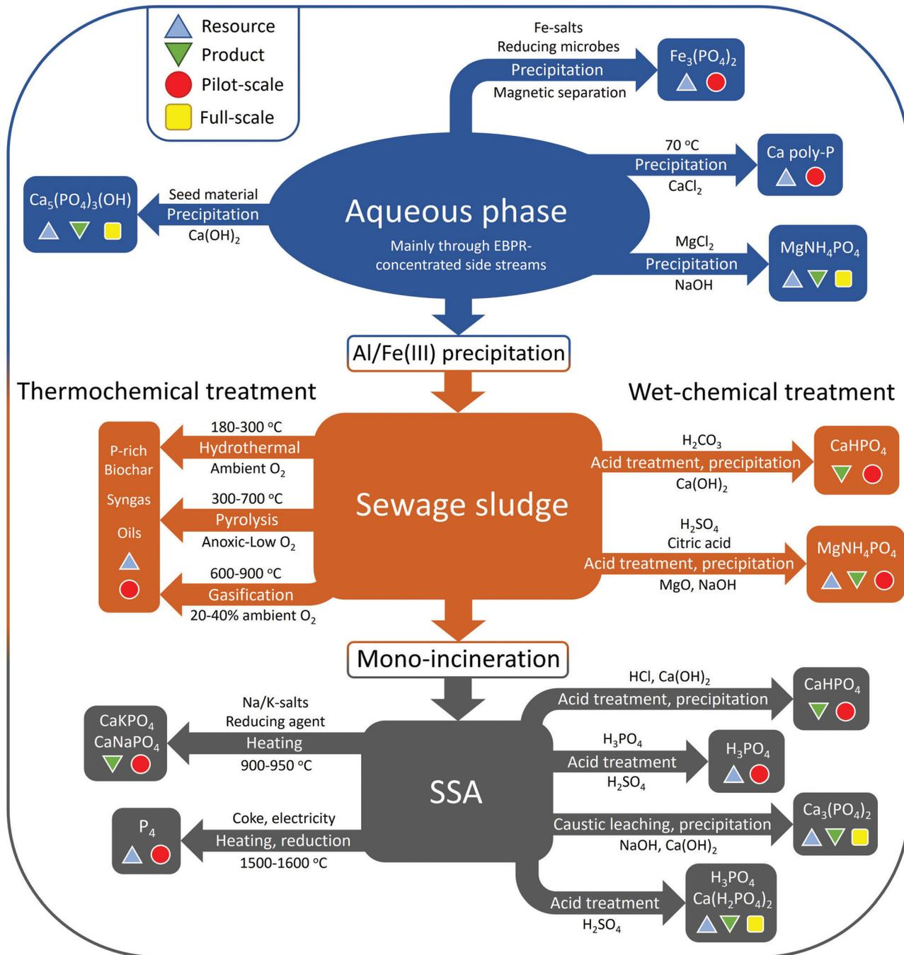
Fig. 4 Schematic overview of P recovery processes.
