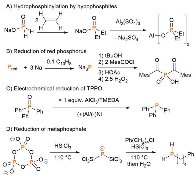
Fig. 3 Selected examples of methods to synthesise organophosphorus compounds avoiding the use of  $\text{PCl}_3$ . Mes = mesityl; OAc = acetate; TPPO = triphenylphosphine oxide; TMEDA = tetramethylethylenediamine.
