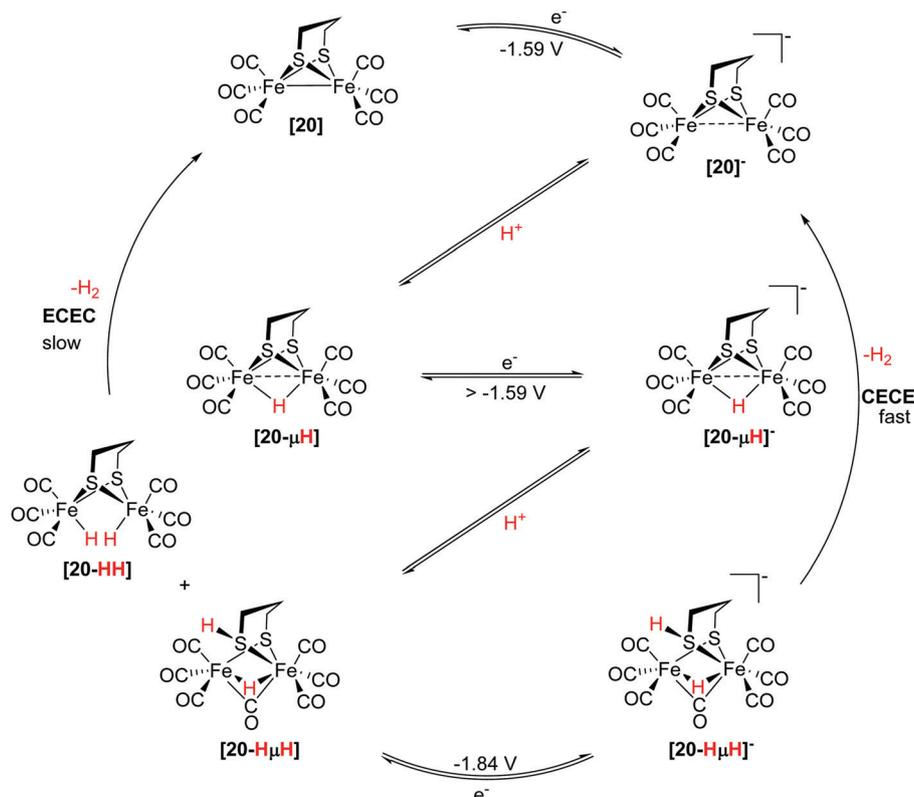
Fig. 98 Catalytic pathway for proton reduction by  $\text{Fe}_2(\text{pdt})(\text{CO})_6$ .
