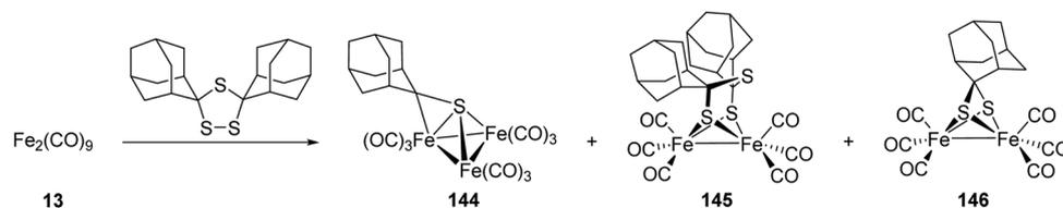
Fig. 42 Synthetic pathways to novel sdt complexes from  $\text{Fe}_2(\text{CO})_9$ .
