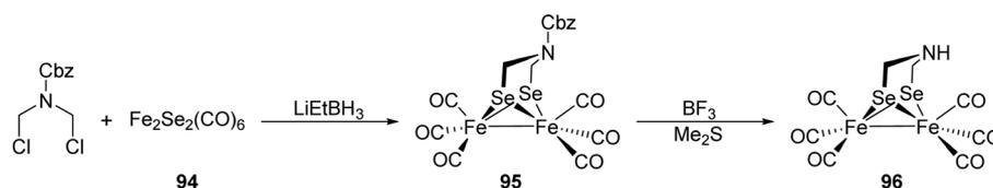
Fig. 34 Synthetic pathway to  $\text{Fe}_2(\text{adSe})(\text{CO})_6$  (**96**).
