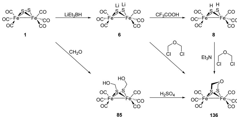
Fig. 40 Synthesis routes towards Fe<sub>2</sub>(odt)(CO)<sub>6</sub>.
