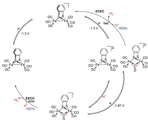
Fig. 100 Catalytic pathway for proton reduction by **149**.
