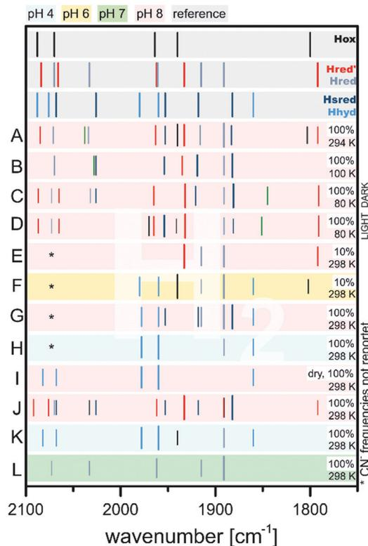
Fig. 11 Schematic representation of IR band positions of  $\text{H}_2$  reduced *CrHydA1* (coloured background) in comparison with currently known states (grey background). IR signatures of known states are taken from Table 2. References for entries: A,<sup>55</sup> B,<sup>60</sup> C and D,<sup>82</sup> E and F,<sup>51</sup> G to I,<sup>75</sup> J and K,<sup>67</sup> L.<sup>72</sup>
