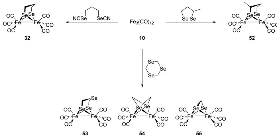
Fig. 28 Synthesis of selenium modified H-cluster models.
