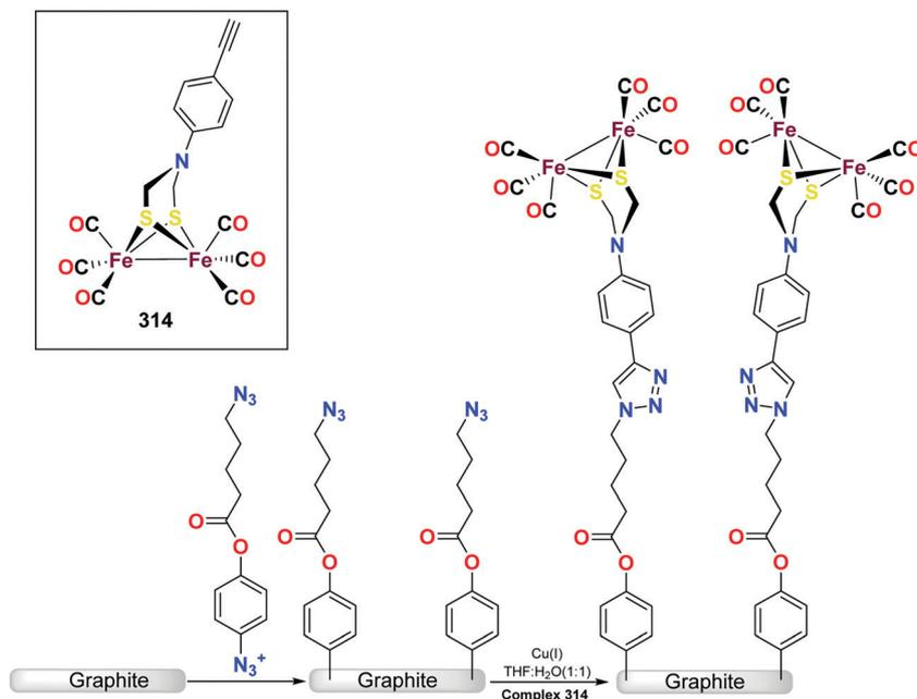
Fig. 107 Schematic presentation of covalent attachment for the [FeFe]-hydrogenase model **314** on modified graphite surfaces. Reproduced from ref. 517 with permission from The Royal Society of Chemistry.
