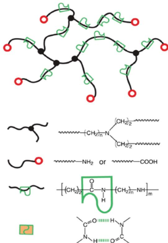
Fig. 32 Schematic representation of the hybrid elastomer produced by Weitz *et al.* Reproduced with permission.<sup>16</sup> Reproduced from ref. 16 with permission from Wiley, copyright 2017.
