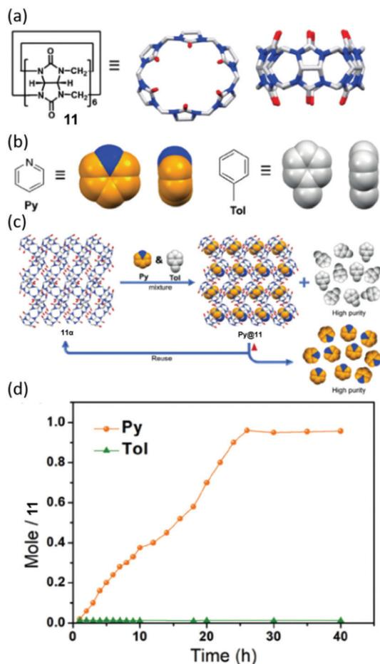
Fig. 28 Chemical structures and cartoon representations of (a) **11** and (b) pyridine and toluene. (c) General scheme showing adsorption and separation of pyridine and toluene by NACs of **11**. (d) Time dependent solid–vapour sorption profile for single component pyridine and toluene vapours, reproduced with permission.<sup>174</sup> Reproduced from ref. 174 with permission from Wiley, copyright 2020.
