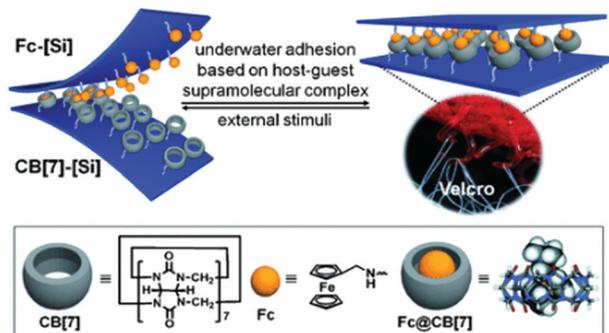
Fig. 36 A schematic representation of the CB[7]/aminomethylferrocene 'velcro', with a light microscope image of traditional hook and loop Velcro.<sup>205</sup> Reproduced from ref. 205 with permission from Wiley, copyright 2013.
