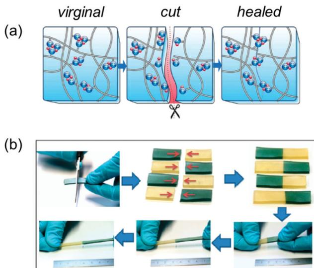
Fig. 34 (a) The movement of charge clusters allowing reformation of the material. (b) The self-healing nature of the material, demonstrated by the use of coloured dye.<sup>198</sup> Reproduced from ref. 198 with permission from the American Chemical Society, copyright 2015.
