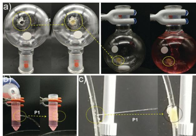
Fig. 38 Compound **22** fixing and making watertight (a) a broken glass round bottom flask, (b) a centrifuge tube and (c) a water pipe.<sup>221</sup> Reproduced from ref. 221 with permission from the American Chemical Society, copyright 2020.
