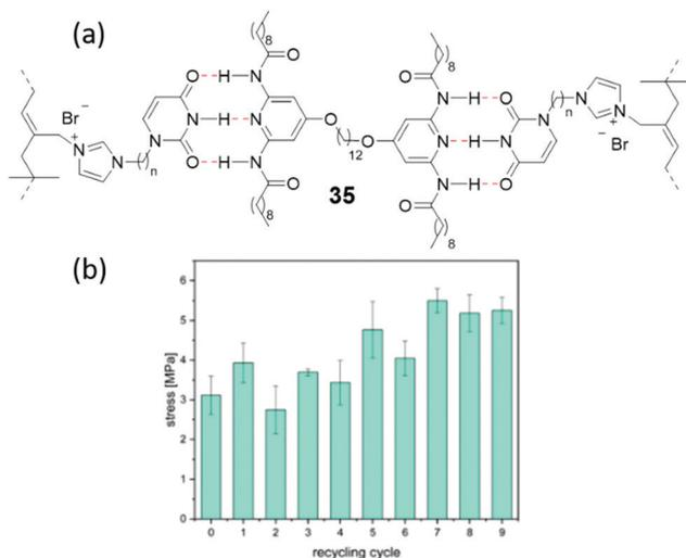
Fig. 35 (a) Ionically modified butyl rubber doped with uracil (**35**) to give hydrogen bonding interactions; red dotted lines indicate hydrogen bonding. (b) Stress at break values after 9 reprocessing cycles.<sup>204</sup> Reproduced from ref. 204 with permission from the Royal Society of Chemistry, copyright 2020.
