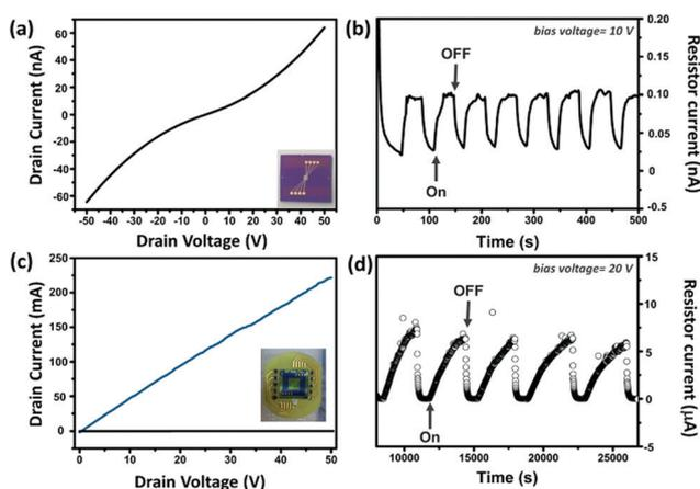
Fig. 42 (a) *I*-*V* curve of the Lp-pi-COF film with tested device shown in photograph. (b) On-off switching behavior upon light irradiation of device from graph (a). (c) *I*-*V* curve of the Lp-pi-COF recorded in argon (black) and water vapor (blue) environment with tested device shown in photograph. (d) On-off switching behavior upon moisture exposure of device from graph (c). Reproduced with permission.<sup>209</sup> Copyright 2018, American Chemical Society.
