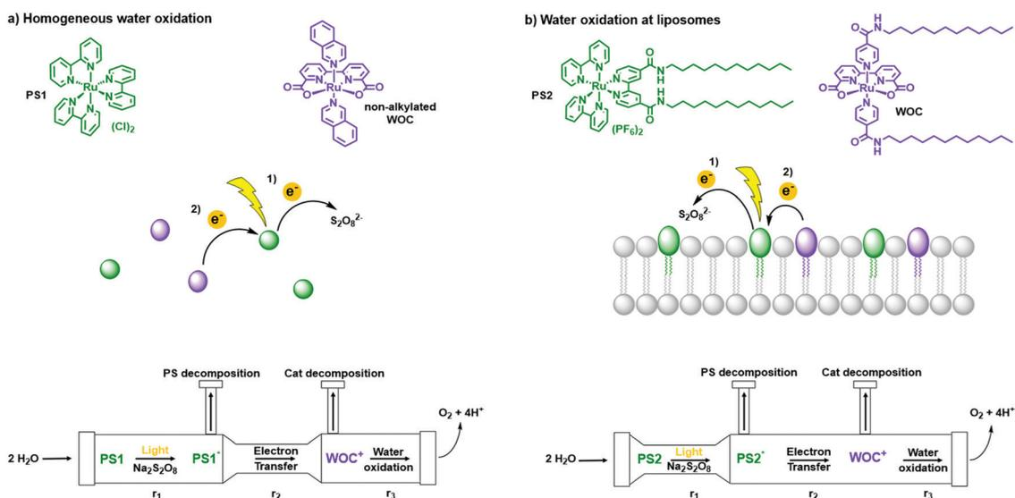
Fig. 16 Water oxidation in (a) homogeneous solution and at (b) liposomes. (top) Photosensitisers (green) **PS1** and **PS2** and catalysts (purple) non-alkylated **WOC** and **WOC**. (middle) Schematic step-by-step electron transfer in homogeneous conditions and at liposomes. (bottom) Scheme of three rate determining steps (RDS) in photocatalytic water oxidation under homogeneous and liposome conditions. Figure adapted with permission from ref. 50.
