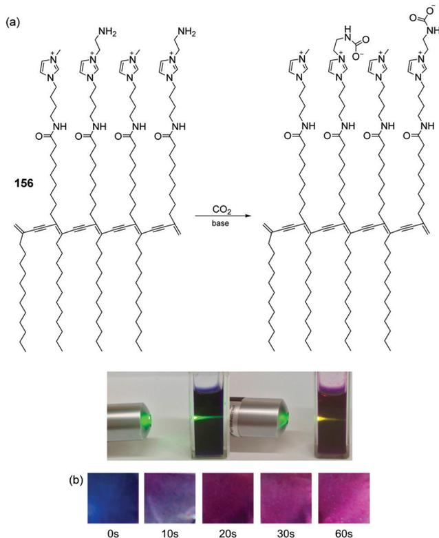
Fig. 15 (a) Structure of **156**, and proposed origin of the CO<sub>2</sub> induced color change. (b) Time-dependent color changes of **156** embedded electrospun microfibers in a CO<sub>2</sub> atmosphere in the presence of saturated TEA vapor.
